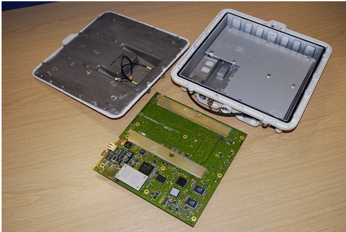
Figure 7: Connectorised version with front antenna connector plate removed.
