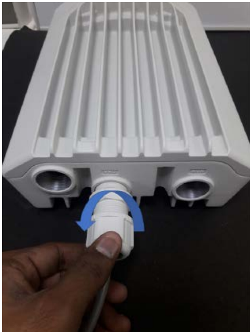
Figure 115: Removing the cable clamp
