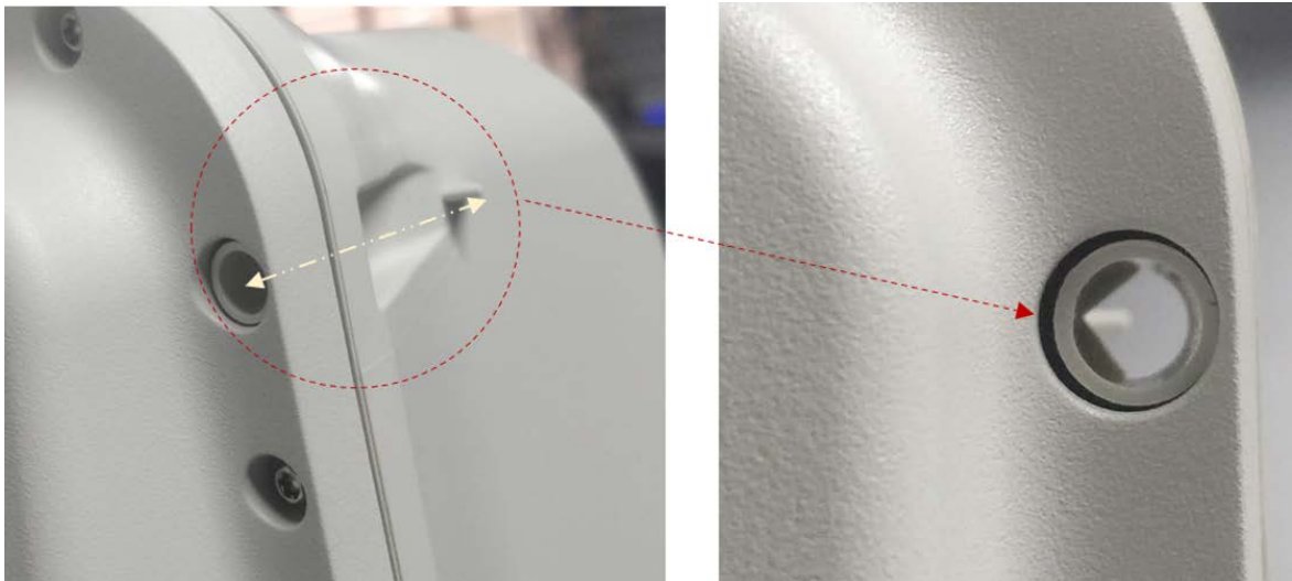
Figure 78: Aligning the V2000 device
