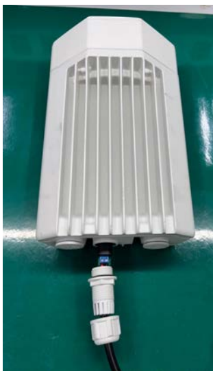
Figure 122: Connecting the input side of AC/DC PSU
