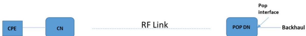
Figure 55: Point to Point cnWave link
