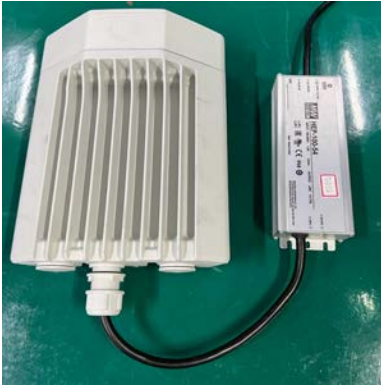
Figure 123: Connecting the output side of AC/DC PSU
