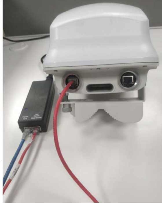
Figure 135: Connecting the V2000 power injector
