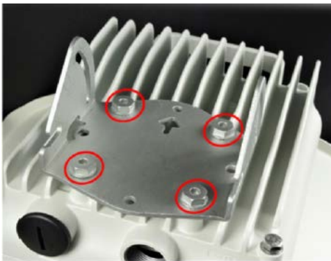
Figure 102: Fixing the mounting plate of the tilt bracket
