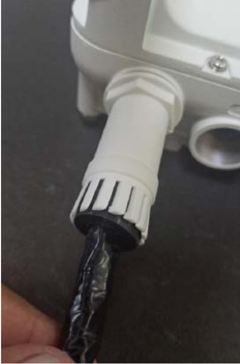
Figure 146: Fitting the gland body
