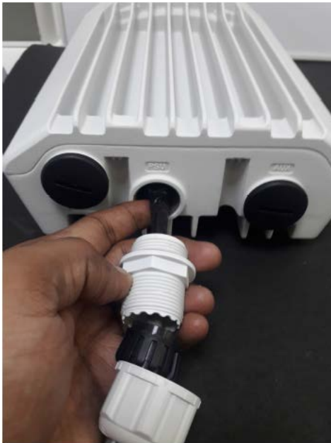
Figure 117: Removing the latch of the RJ45 plug
