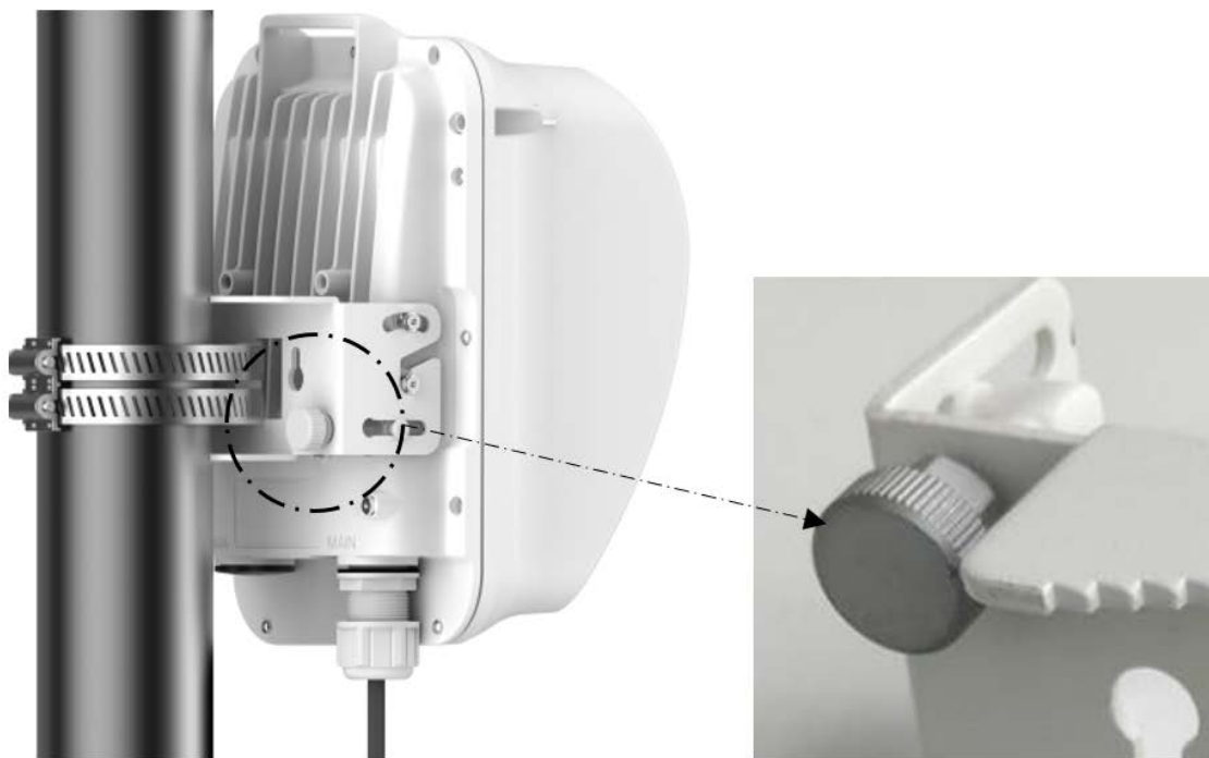
Figure 80: Using the adjustable bracket knob for alignment
