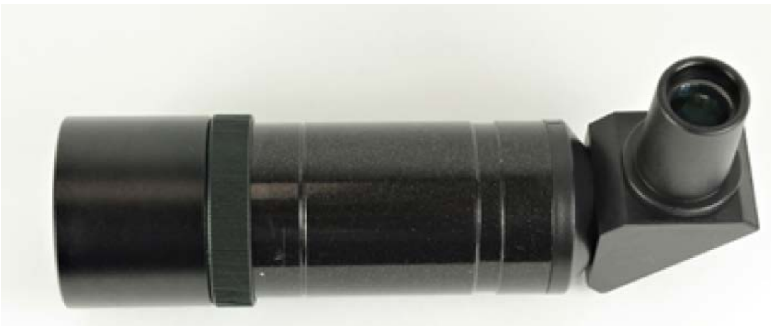
Figure 27: Typical alignment telescope
