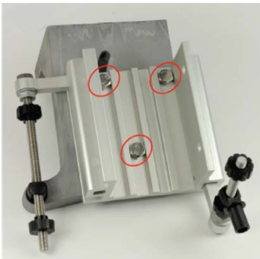
Figure 84: MB Screws in the slots in the bracket base
