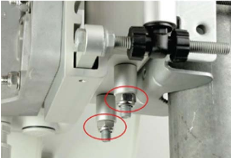
Figure 94: Two Nyloc screws in the azimuth
