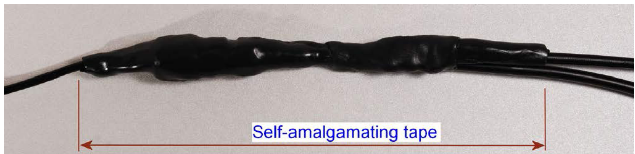
Figure 122 Wrapping self-amalgamating tape around the GPS adapter cable joint
