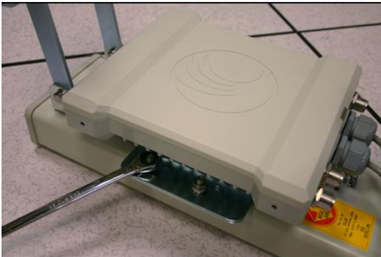
Figure 83 Lower bracket attached to AP antenna
