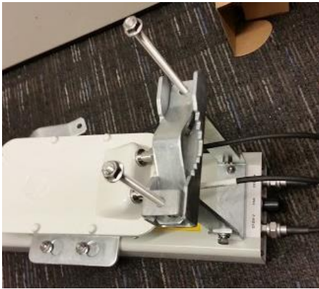
Figure 73 Lower bracket attached to AP antenna
