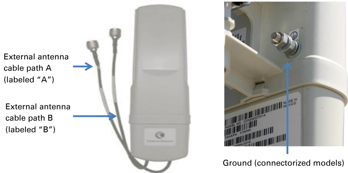
Figure 5 PMP/PTP 450 Series – SM/BH Connectorized interfaces
