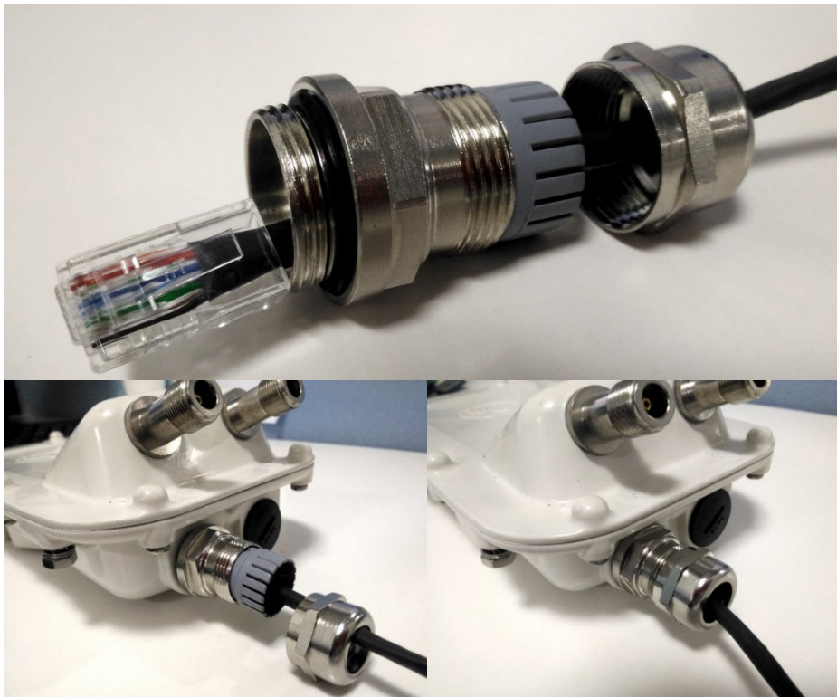
Figure 123 Ethernet cable gland for PMP/PTP 450i Series
