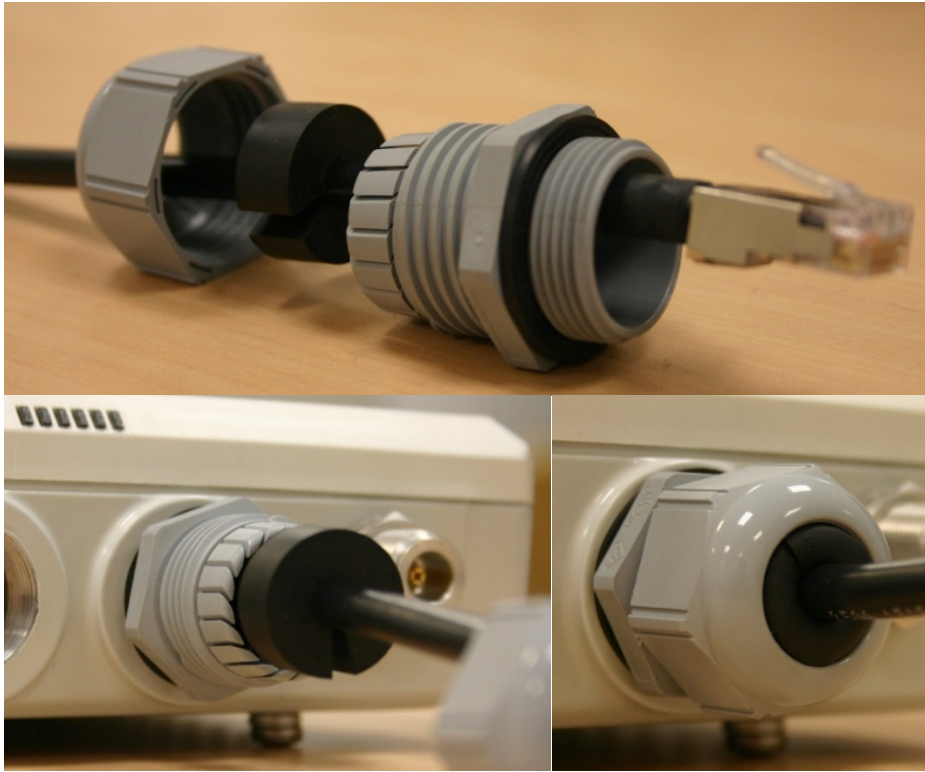
Figure 122 Ethernet cable gland for PMP/PTP 450 Series
