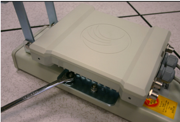
Figure 102 Lower bracket attached to AP antenna
