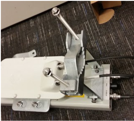
Figure 92 Lower bracket attached to AP antenna
