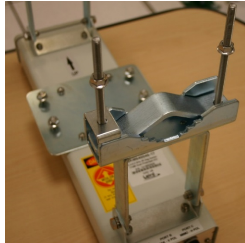
Figure 101 Attaching bracket to the rear of the AP
