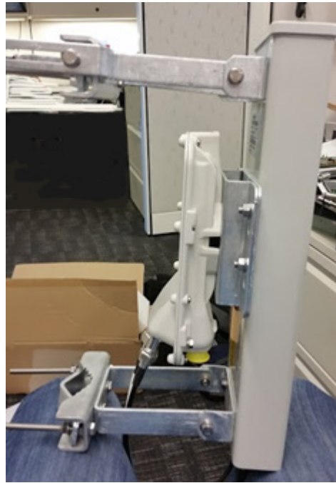
Figure 95 Completed AP and antenna assembly
