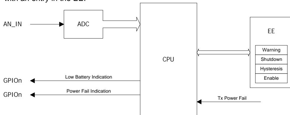
Given that the monitoring functions have been enabled, the signals associated with these functions can be selectively enabled on any of the GPIO pins on the interface connector. Obviously, if the associated signals with this feature are not provided on the interface, external devices will not see any of the warnings and must simply identify when the modem has shutdown.
