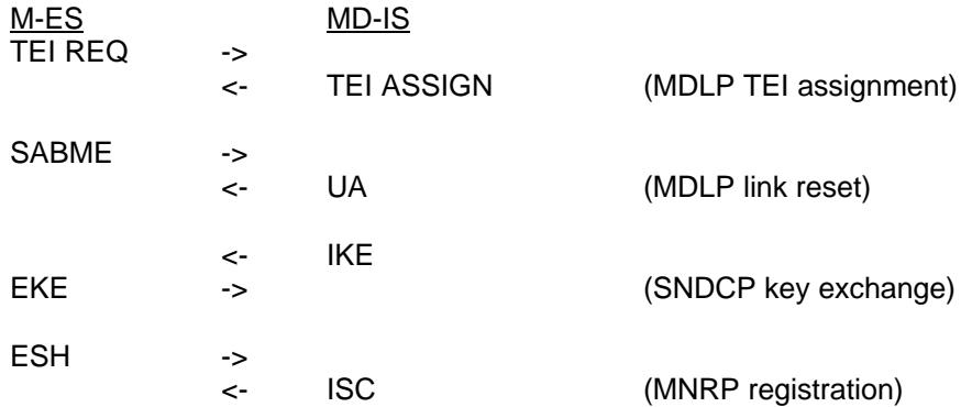
This is the system's response to a registration request, and is basically an accept or deny (refer to Table 507-6 in the CDPD specification for all possible responses). The modem will simply pass the information ("insufficient credentials" in this case) along to the user.
