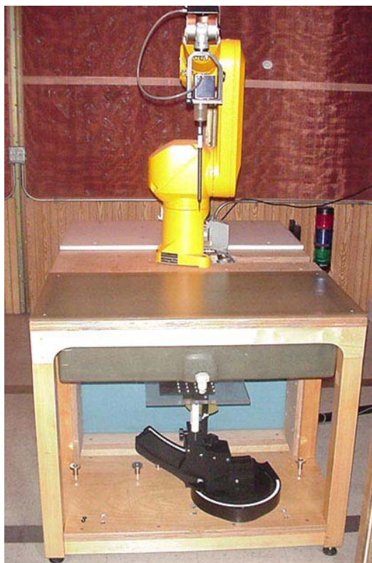
DASY4 SAR Measurement System with planar phantom
