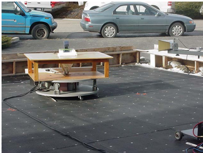
Photograph I.7-1 - 3m EIRP Field Strength Setup
