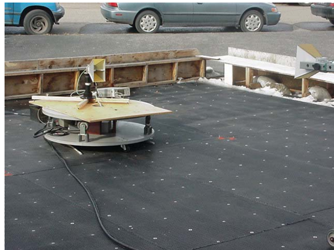
Photograph I.7-2 - 3m EIRP Substitution Setup
