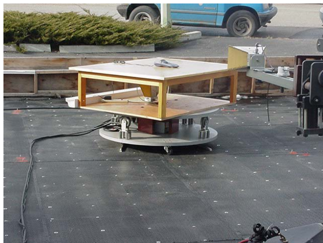
Photograph E.7-3 - 1m Horn/LNA Setup
