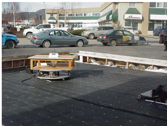
Photograph J.7-4 - 18-26 GHz 1m Horn/LNA Setup
