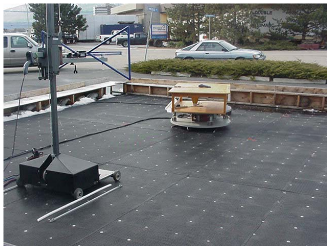
Photograph D.7-1 - 3m ERP Field Strength Setup
