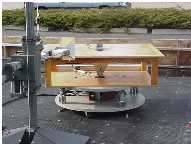
Photograph E.7-3 - 1m Horn/LNA Setup
