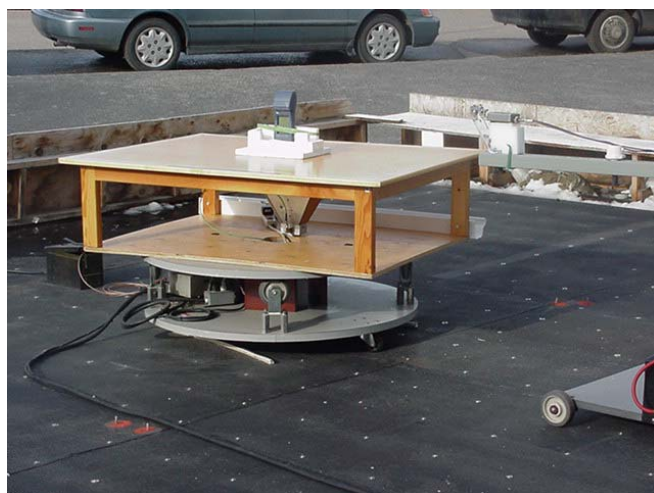
Photograph J.7-4 - 18-26 GHz 1m Horn/LNA Setup
