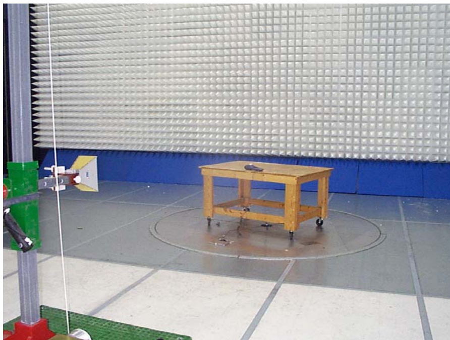
Figure 9-4 FCC §15.109 Test Configuration Photograph
