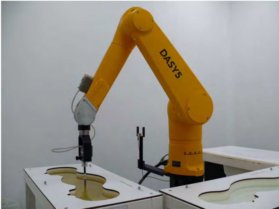
Picture 2: Specific Absorption Rate Test Layout
