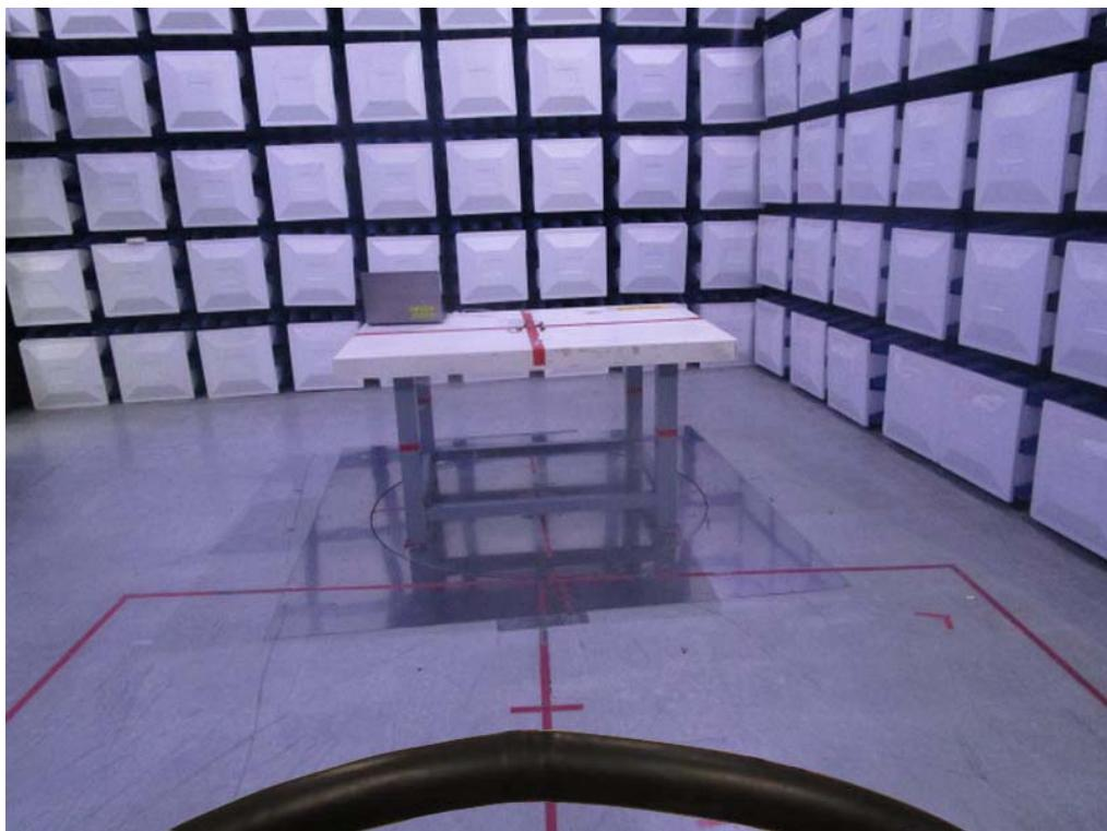
**Radiated Emissions Test Photos****30 MHz to 1000 MHz**
