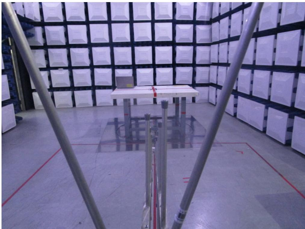
**Radiated Emissions Test Photos****Above 1 GHz**
