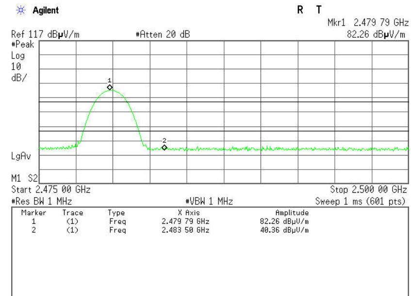
**Detector mode: Average****Polarity: Vertical**
