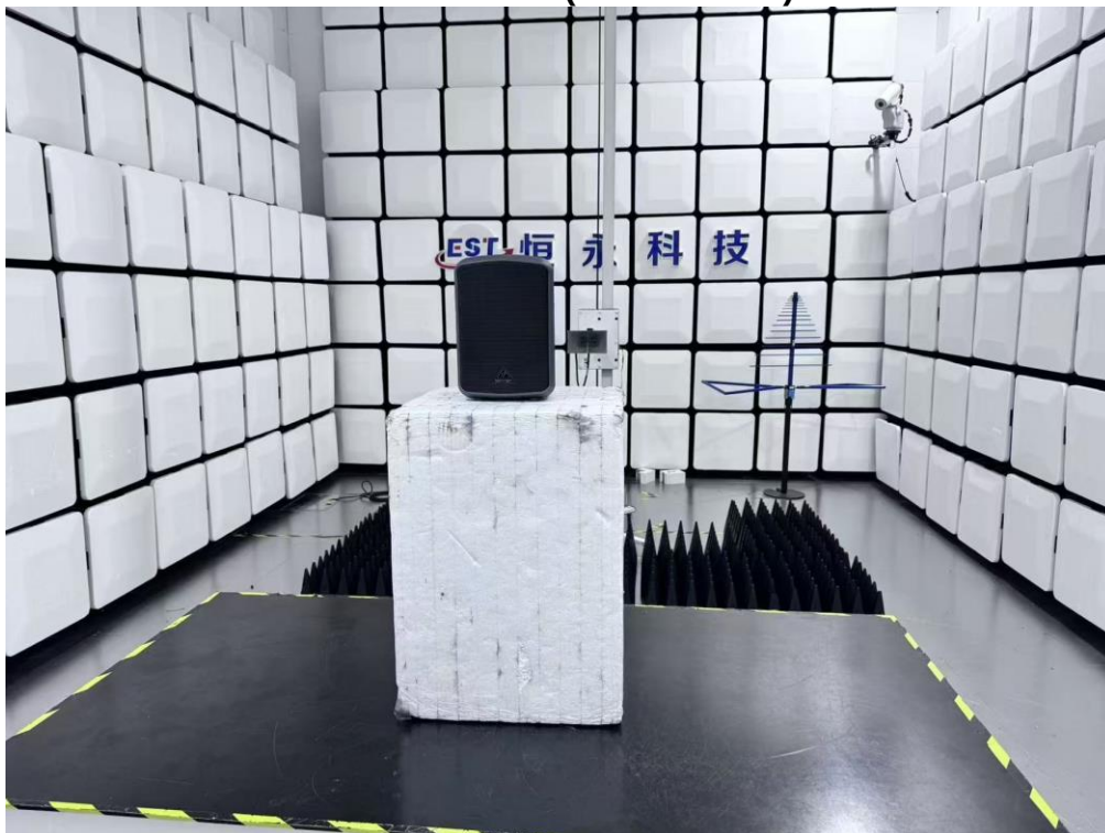
Radiated Test (Above 1GHz)
