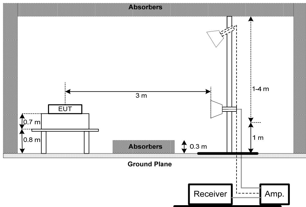
(C) For radiated emissions below 30MHz
