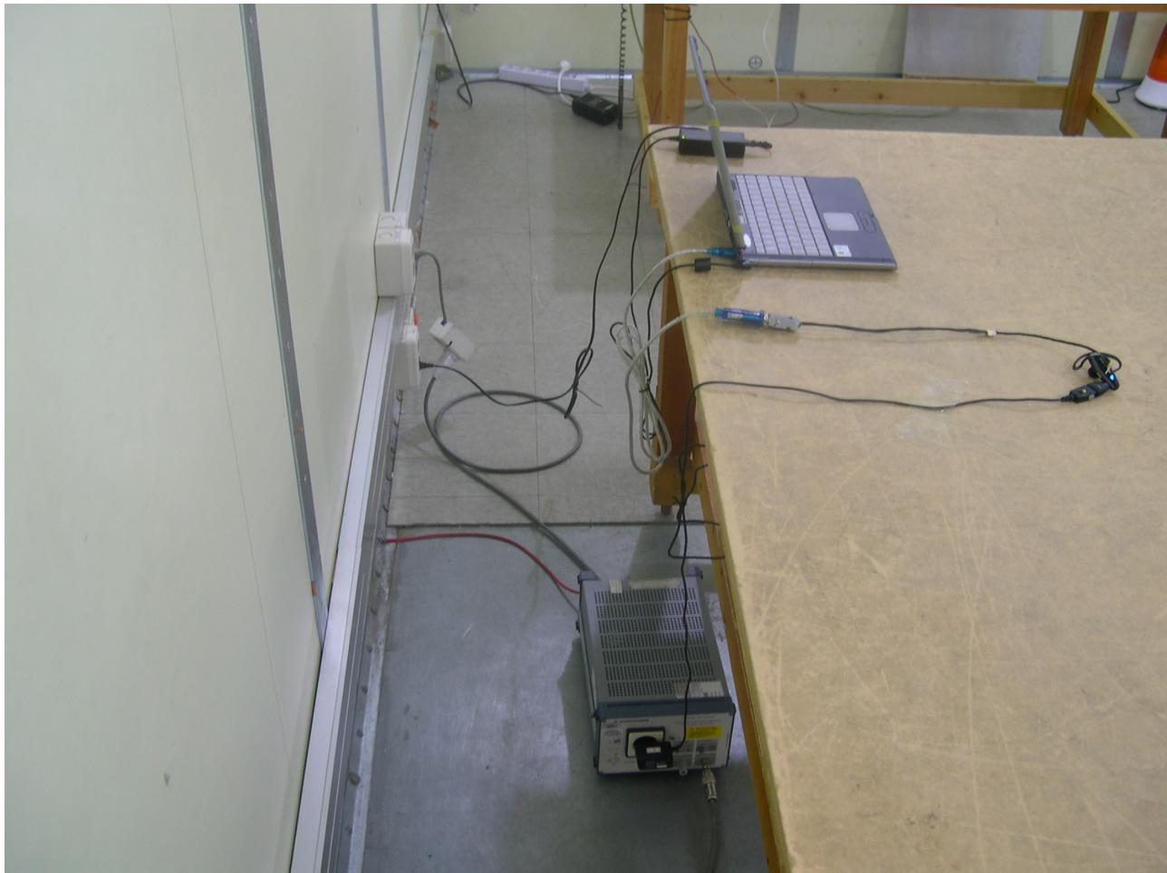
AC power line conducted emission measurement for AC/DC Adaptor #1;
