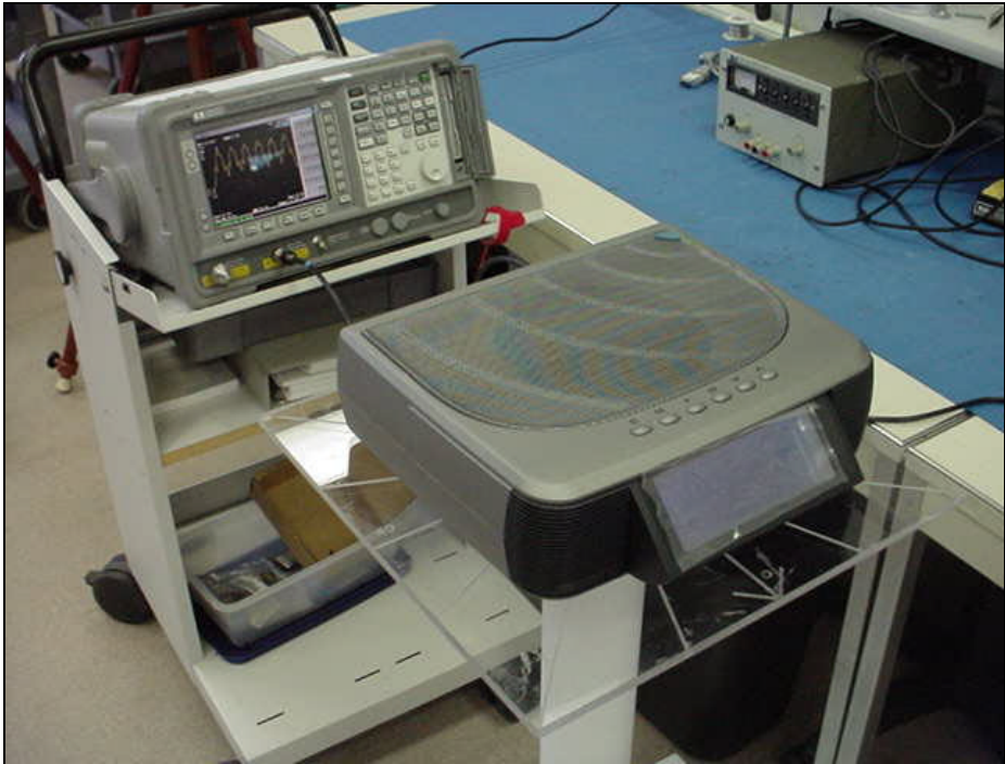
View of Test Setup During the Conducted RF measurements, Table-Top Unit
