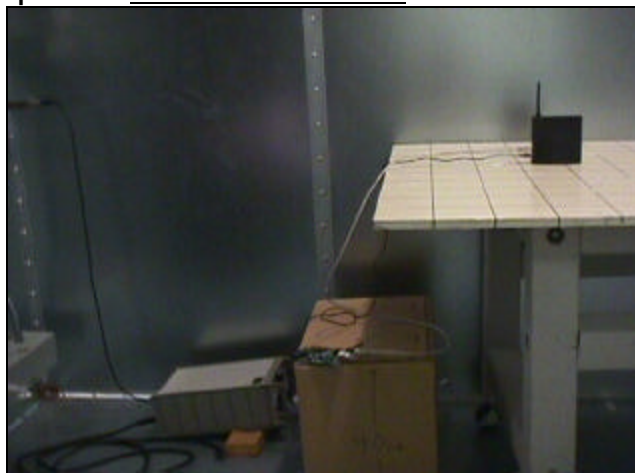
Setup for the Conducted Emissions Test on the Base Unit:
