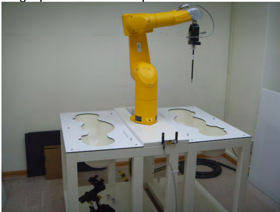
Fig.1 Photograph of the SAR measurement System
