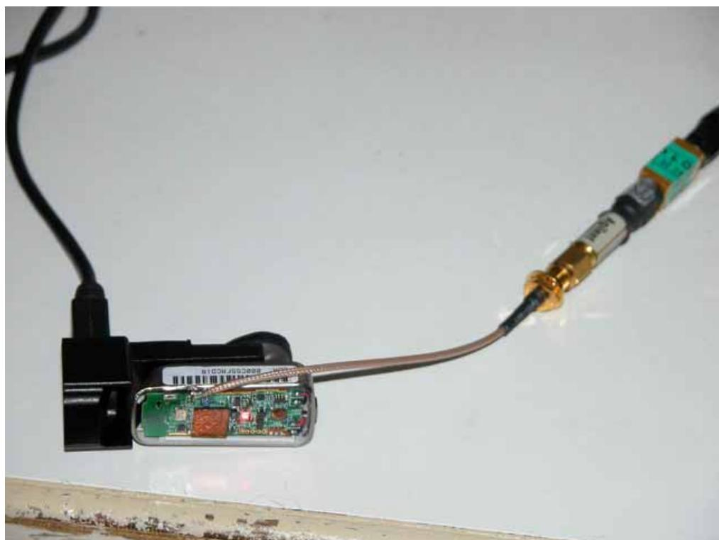
**POWERLINE CONDUCTED EMISSIONS MEASUREMENT SETUP**
