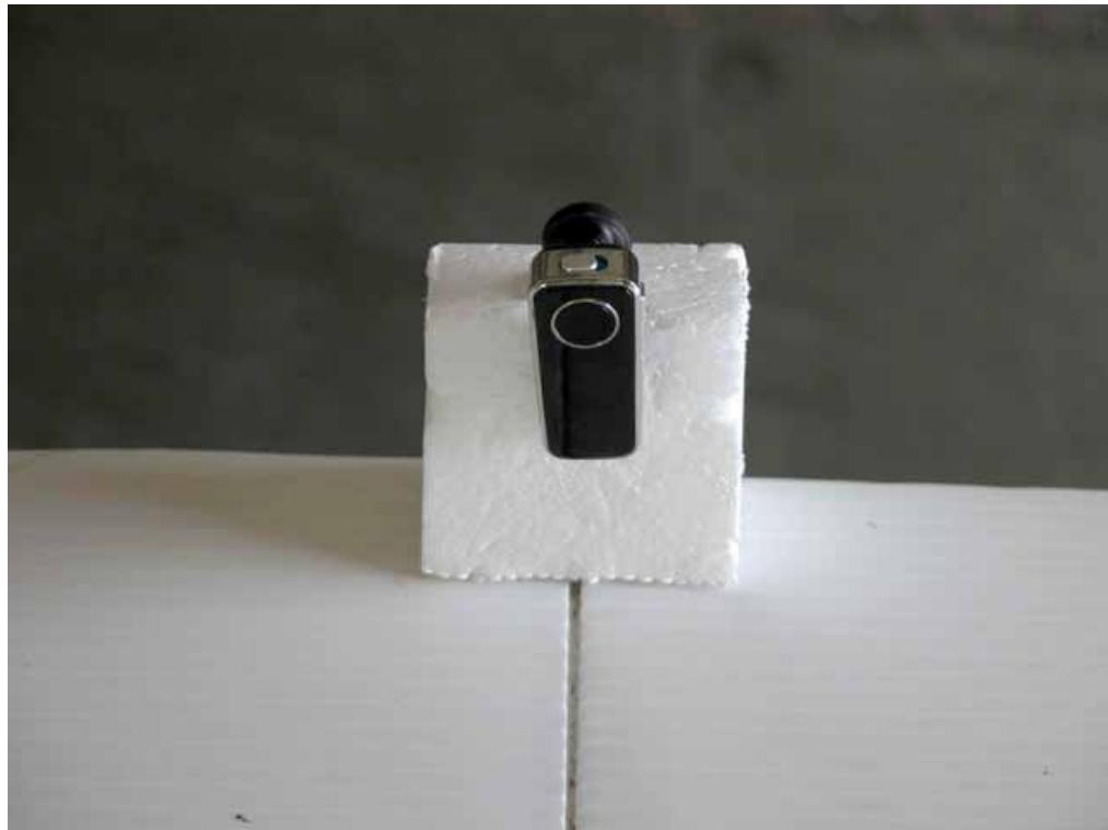
**RADIATED RF MEASUREMENT SETUP**
