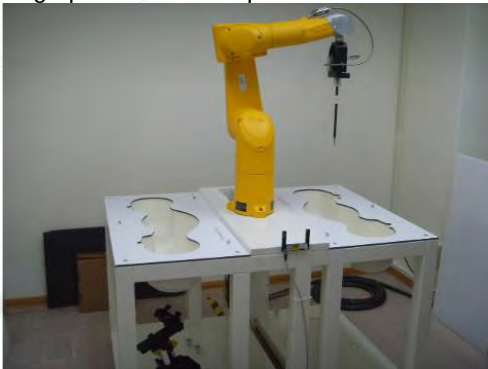
Fig.1 Photograph of the SAR measurement System
