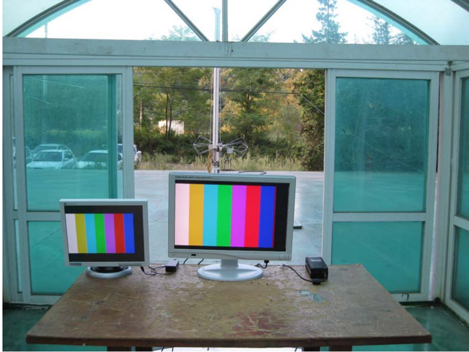
Radiated emission test setup, SDI In, Out Mode, 30MHz to 1GHz, rear
