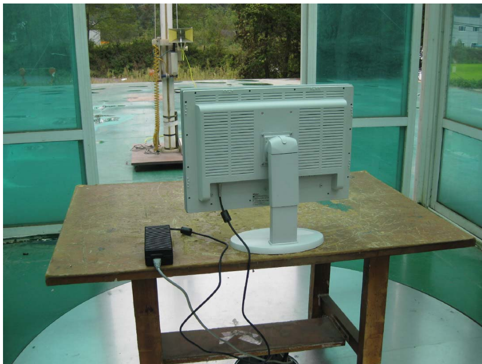
Radiated emission test setup, Standby Mode, 1GHz to 2GHz, rear
