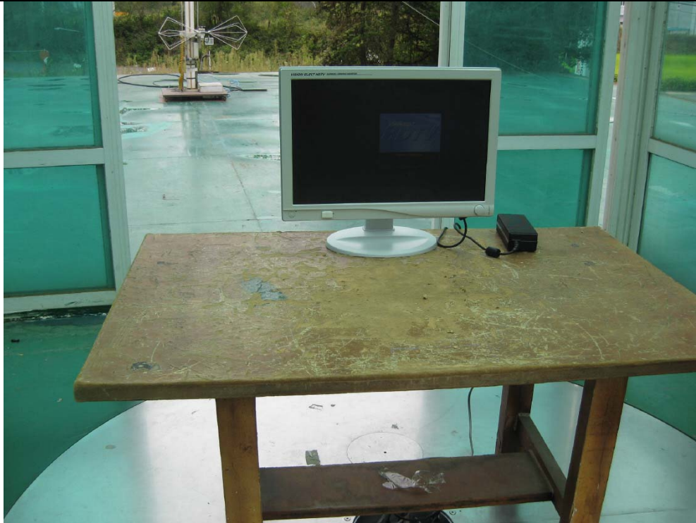
Radiated emission test setup, Standby Mode, 30MHz to 1GHz, rear
