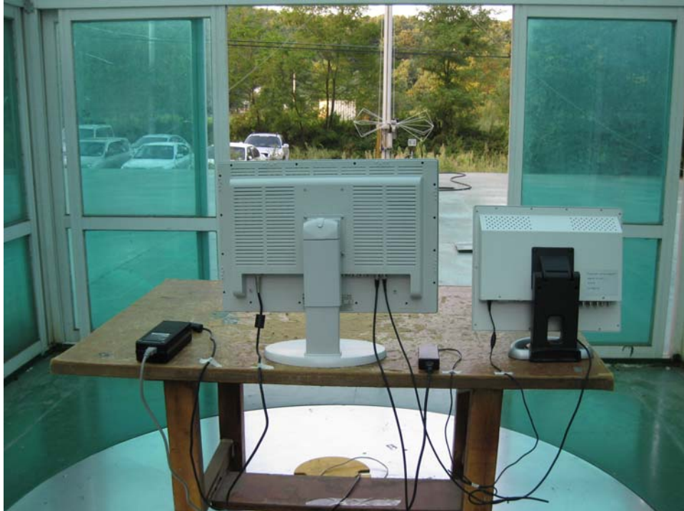
Radiated emission test setup, SDI In, Out Mode, 30MHz to 1GHz, rear
