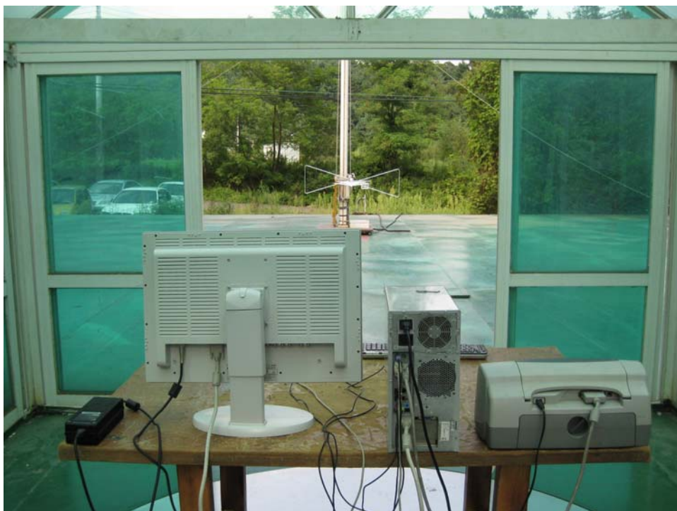
Radiated emission test setup, DVI Mode, 30MHz to 1GHz, rear
