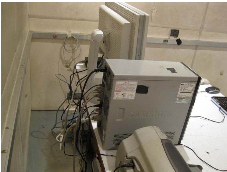
Conducted Emission Test Setup, DVI Mode, side
