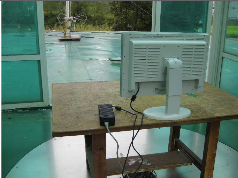
Radiated emission test setup, Standby Mode, 30MHz to 1GHz, rear
