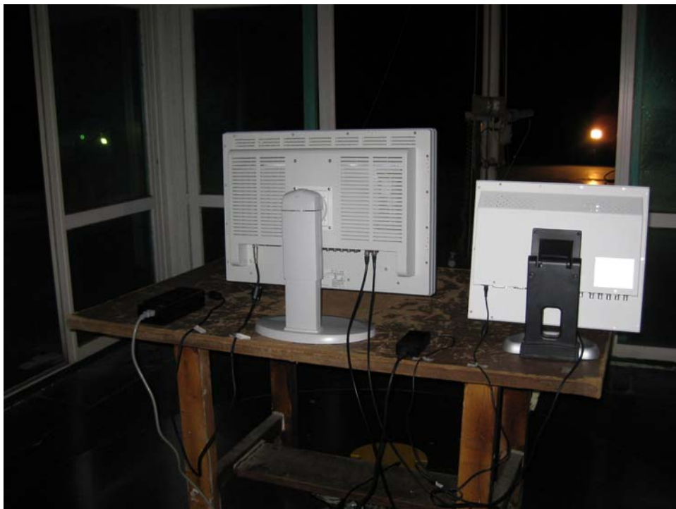
Radiated emission test setup, SDI In, Out Mode, 1GHz to 2GHz, rear
