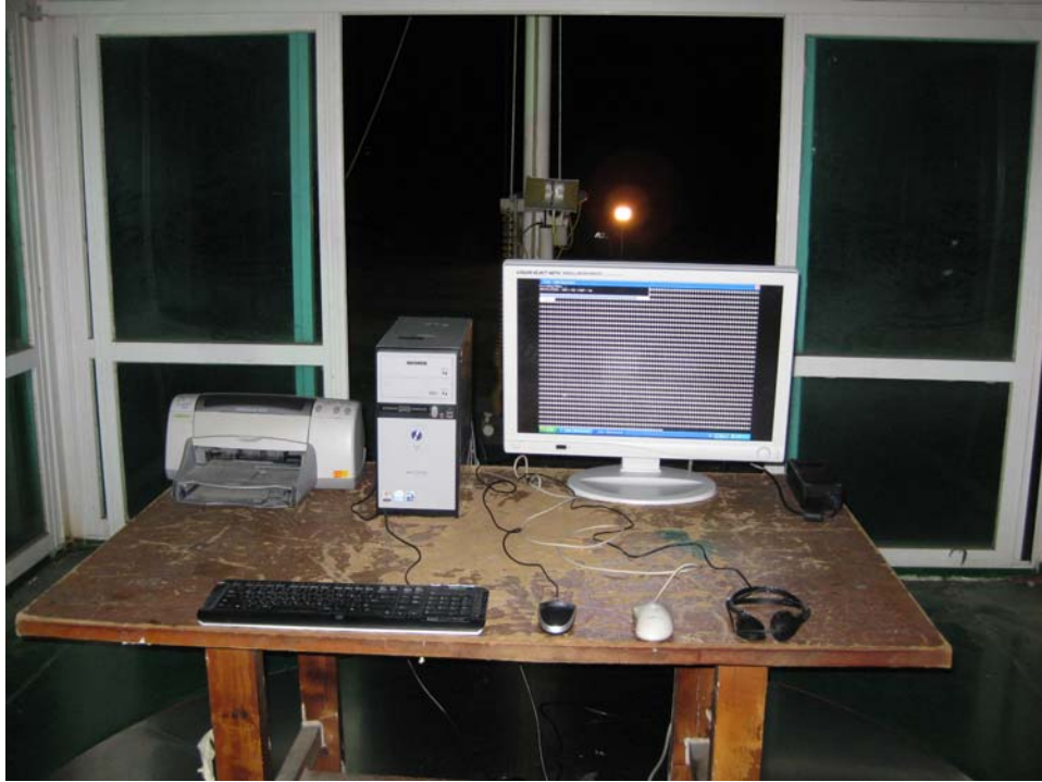
Radiated emission test setup, DVI Mode, 1GHz to 2GHz, rear
