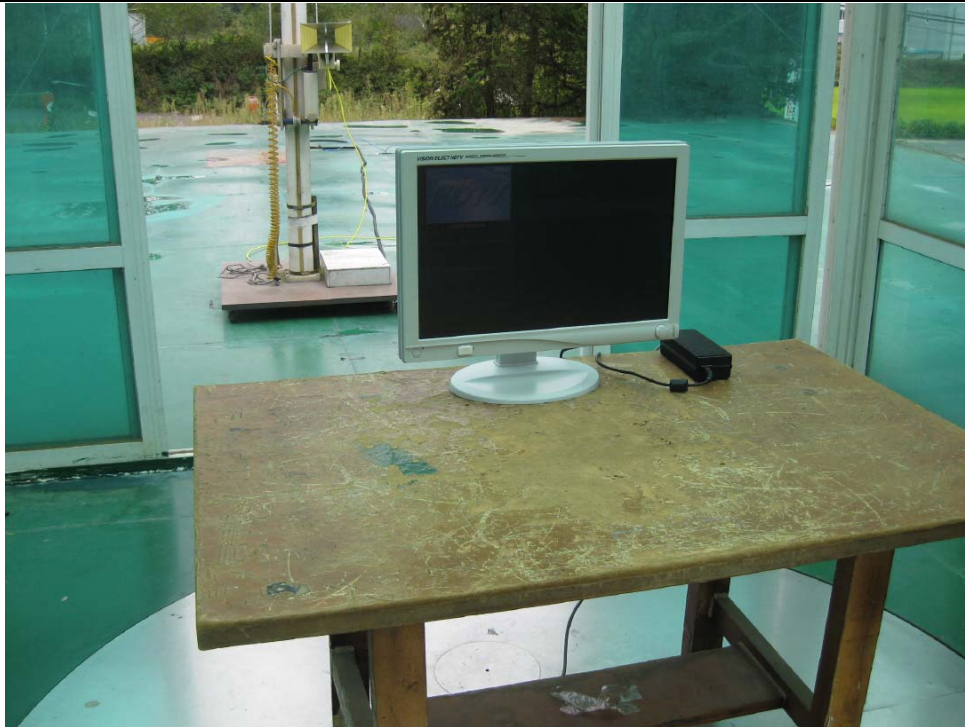
Radiated emission test setup, Standby Mode, 1GHz to 2GHz, rear
