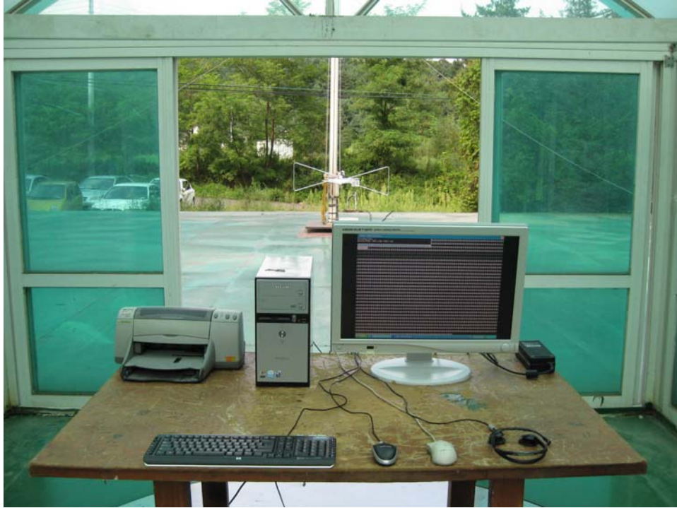
Radiated emission test setup, DVI Mode, 30MHz to 1GHz, rear
