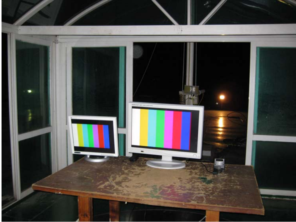
Radiated emission test setup, SDI In, Out Mode, 1GHz to 2GHz, rear
