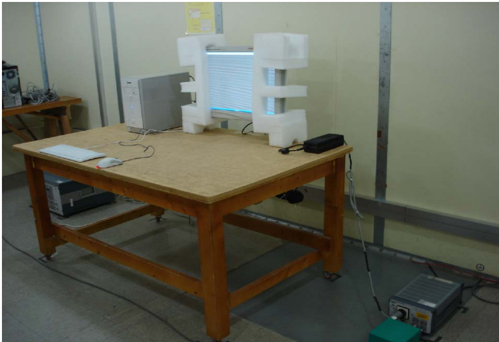
Figure 1. Test Setup for Conducted Emissions (DVI mode)
