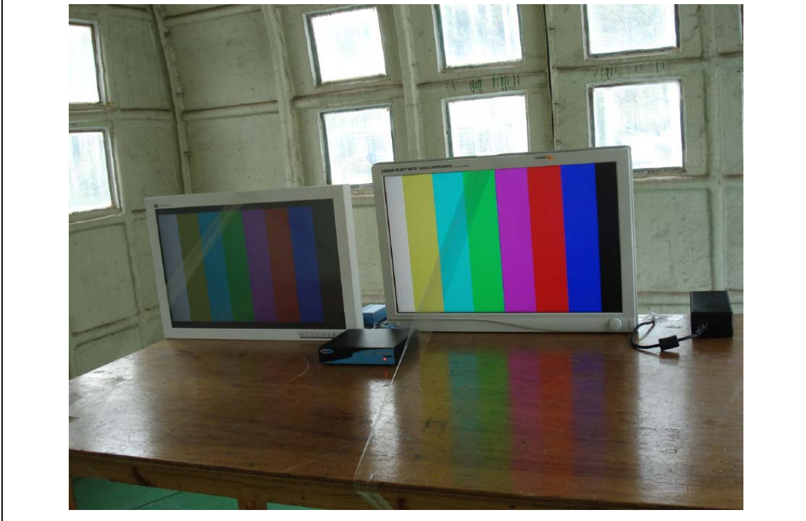
Figure 4. Test Setup for Radiated Emission (SDI Mode)
