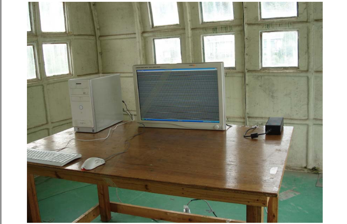
Figure 3. Test Setup for Radiated Emission (DVI Mode)
