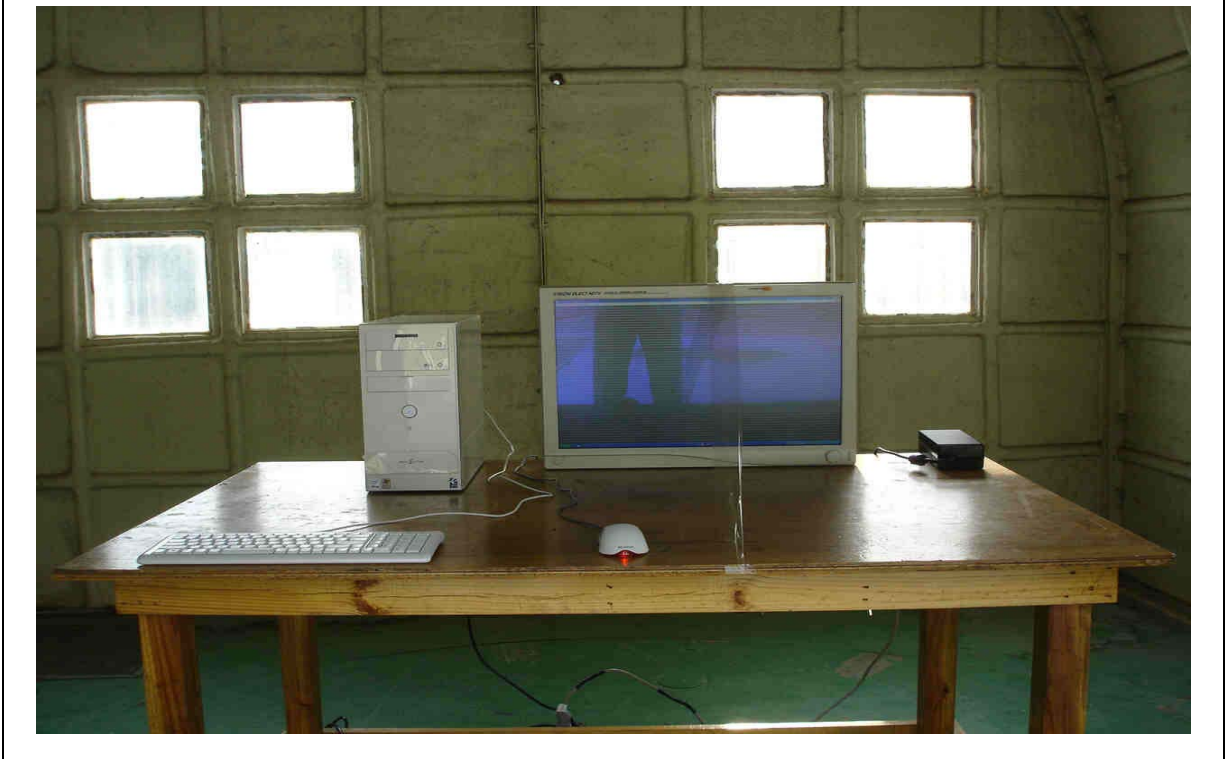
Figure 5. Test Setup for Radiated Emission (VGA Mode)
