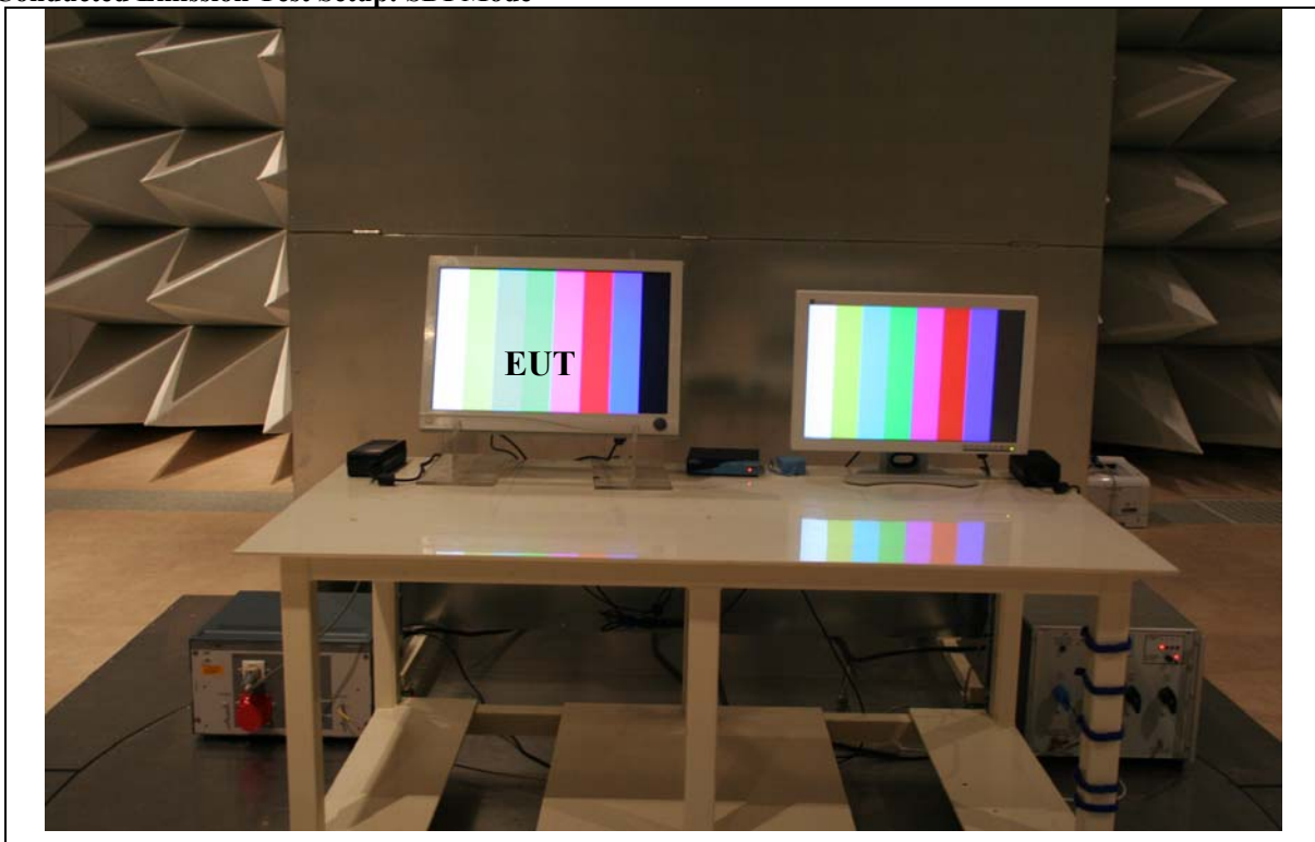
Figure 2 Conducted Emission Test Setup: SDI Mode
