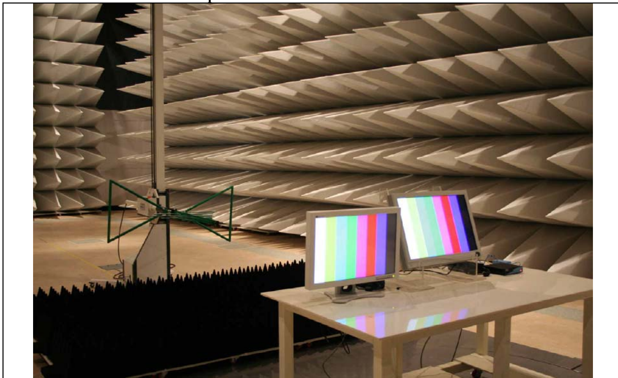
Photo of Radiated emission test setup: 1GHz to 2GHz
