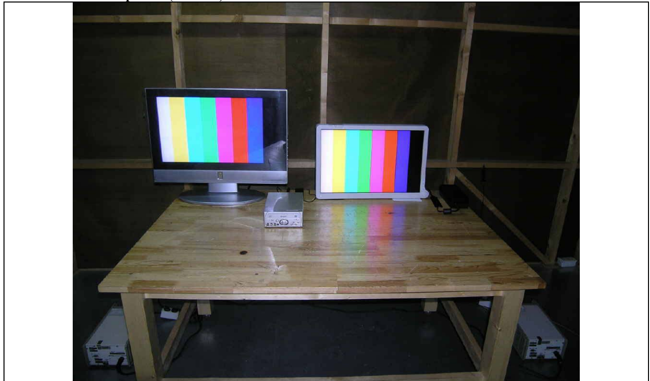
Figure 2. Conducted Emission Test Setup Test Condition: Component (Y/Pb/Pr) In/Out Mode
