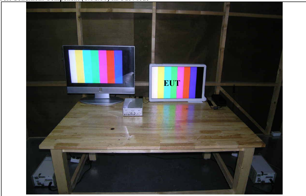
Figure 2 Test Condition: Component (Y/Pb/Pr) In/Out Mode
