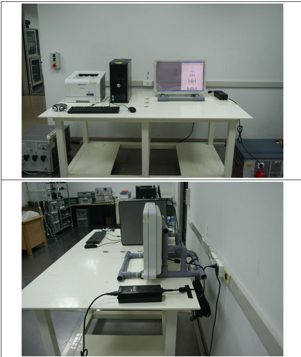
Figure 1. Conducted Emission Test Setup for DVI Mode:
