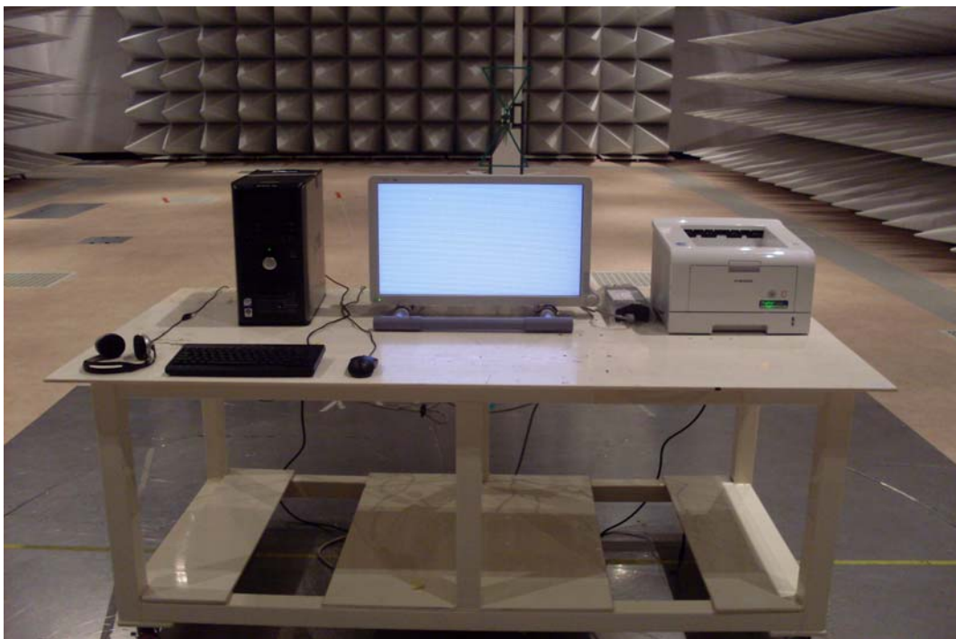
Figure 9, Radiated emission test setup for Test Configuration 1
