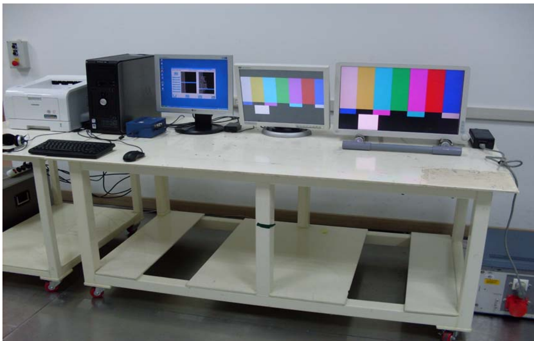
Figure 3. Conducted Emission Test Setup for Test Configuration 1
