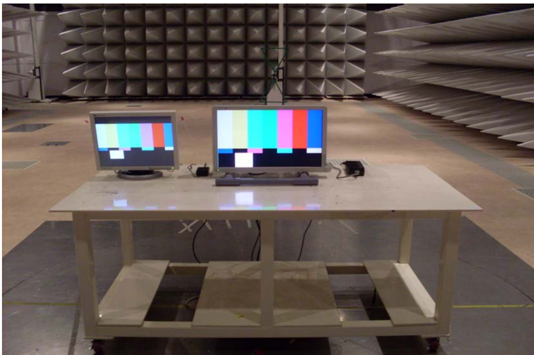
Figure 15, Radiated emission test setup for Test Configuration 2
