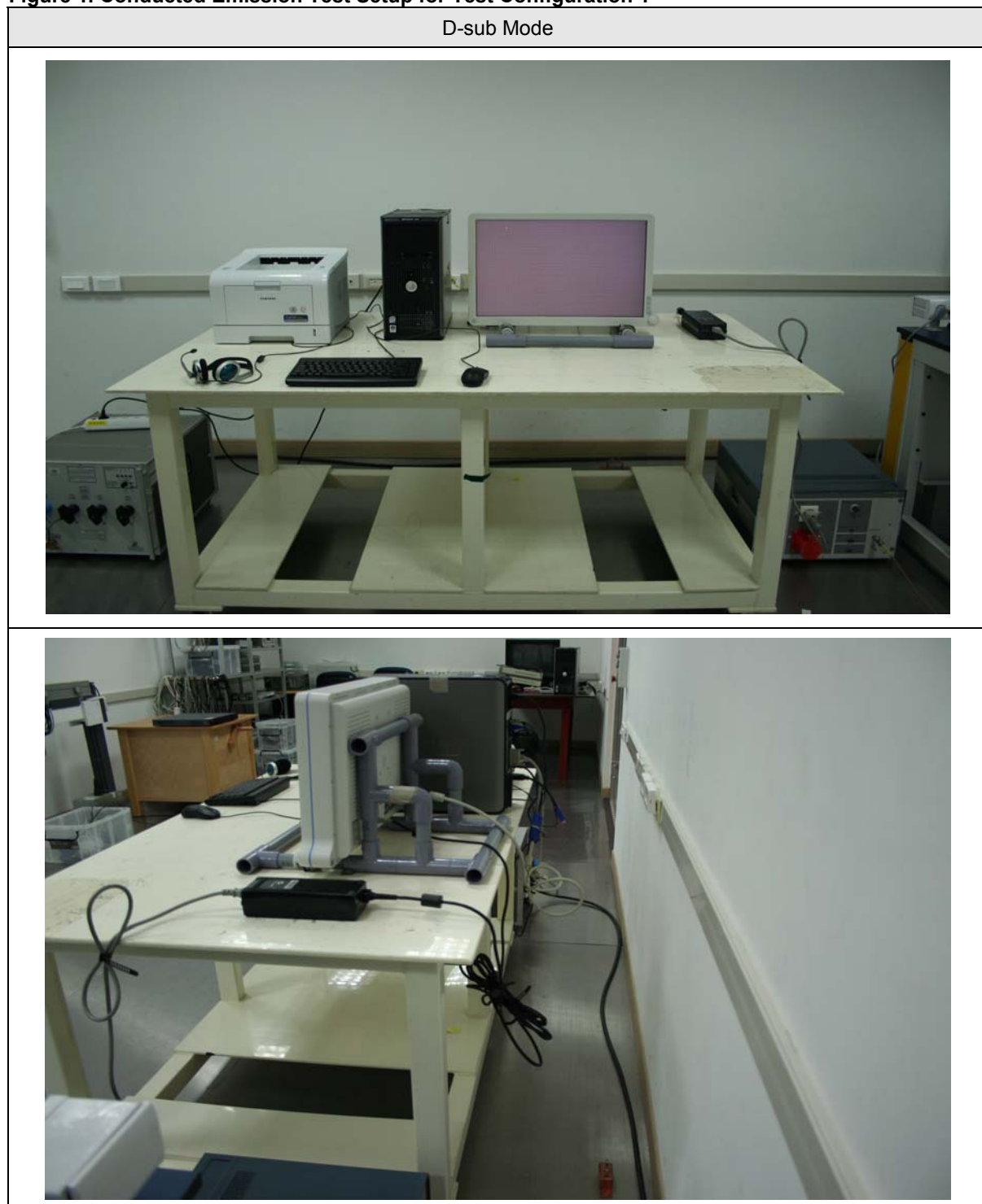
Figure 1. Conducted Emission Test Setup for Test Configuration 1
