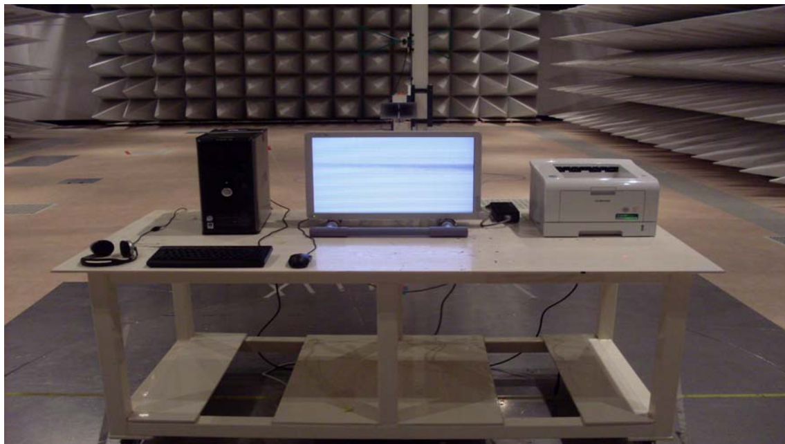
Figure 9, Radiated emission test setup for Test Configuration 2
