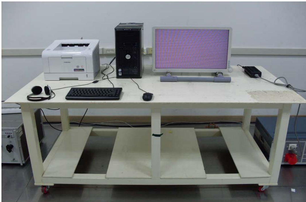
Figure 5. Conducted Emission Test Setup for Test Configuration 2
