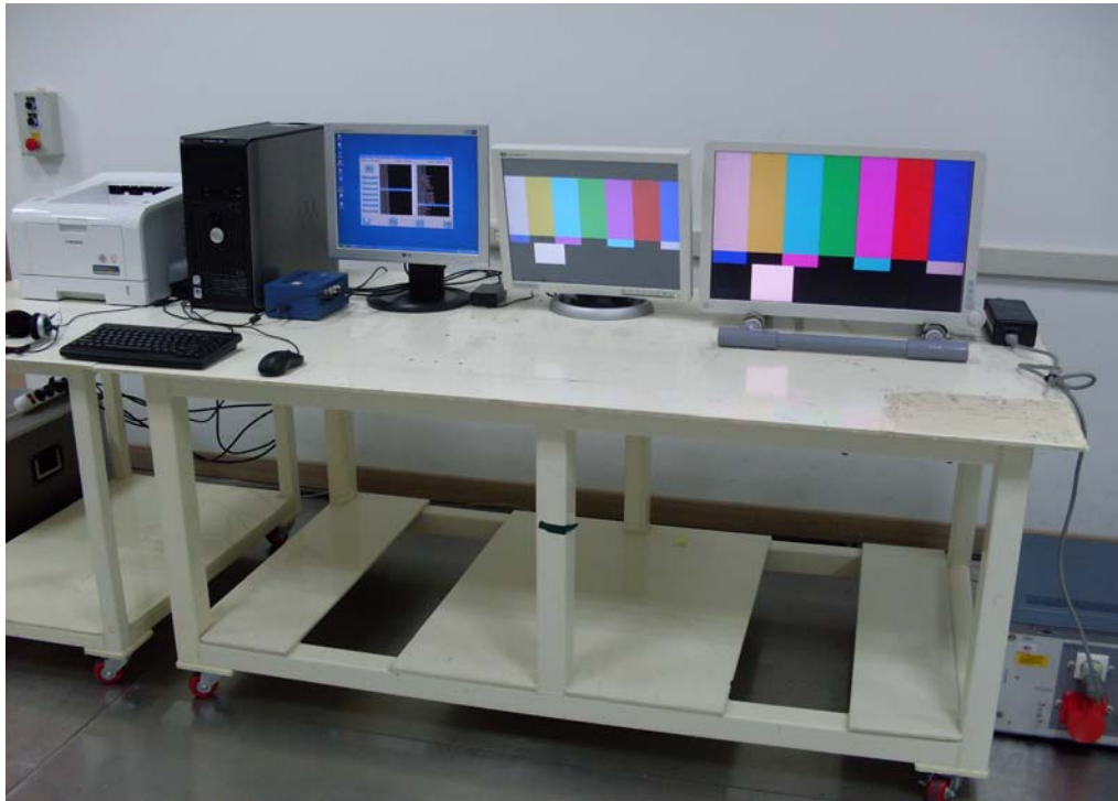
Figure 7. Conducted Emission Test Setup for Test Configuration 2
