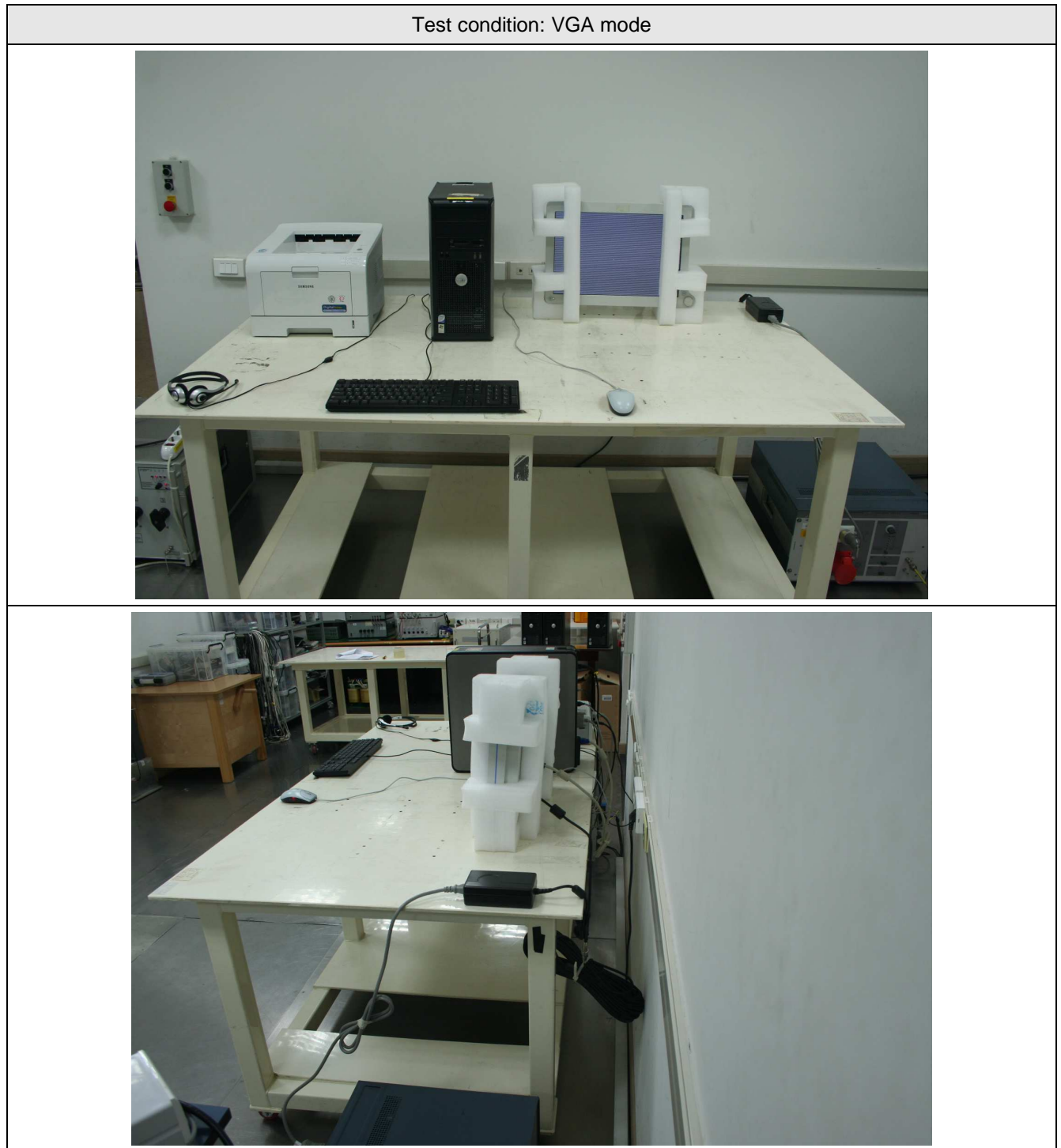
Figure 1. Conducted Emission Test Setup
