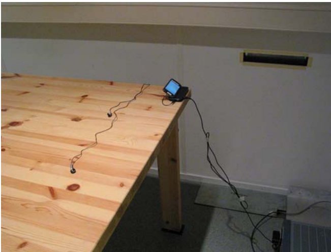
Picture 3 AC powerline conducted emission measurement 15C
