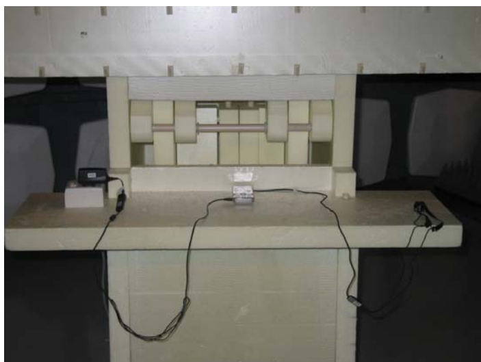
Picture 2 Radiated emission measurement GSM RX / Bluetooth TX
