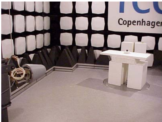
The Anechoic Chamber
