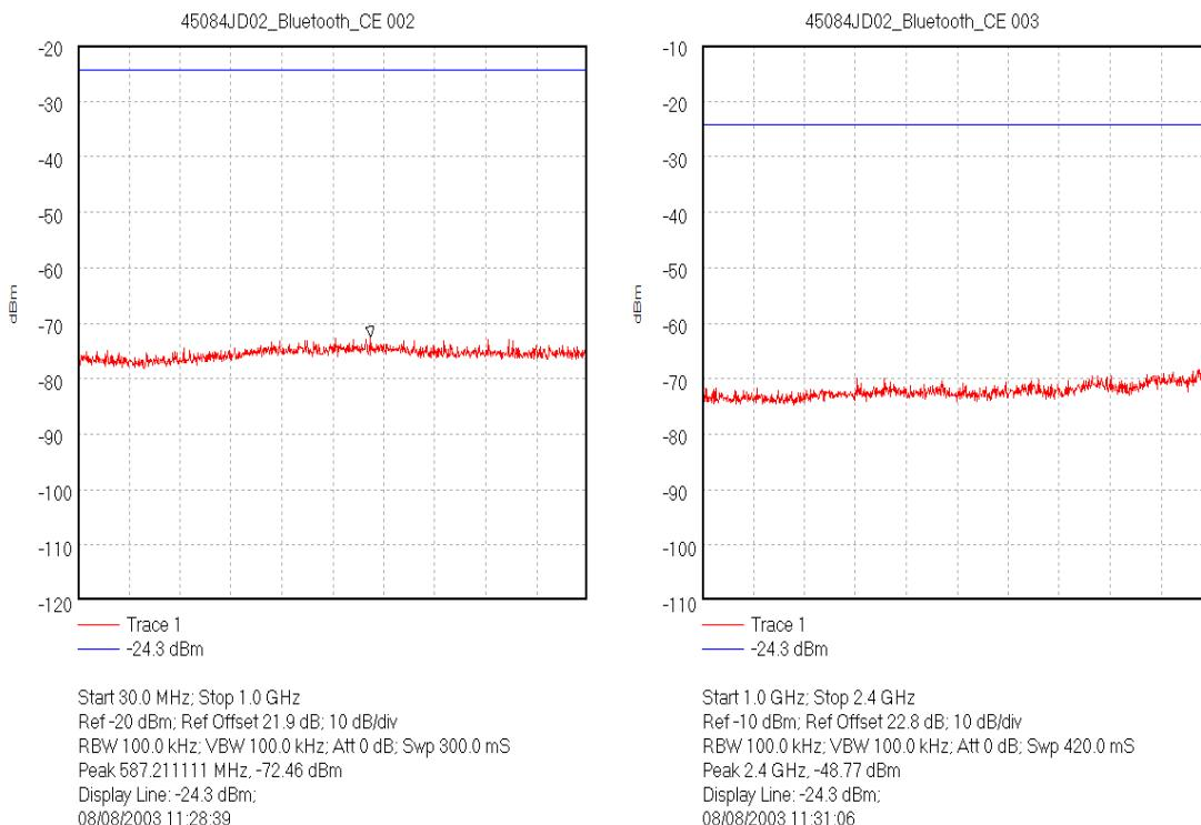
**RADIO FREQUENCY INVESTIGATION LTD****Operations Department****Test Of: Nokia UK Ltd.****NHL-10****To: FCC Part 15.247****TEST REPORT****S.No. RFI/MPTB1/RP45084JD02A****Page 30 of 62****Issue Date: 01 September 2003****Transmitter Conducted Emissions Bottom Channel (Continued)**
