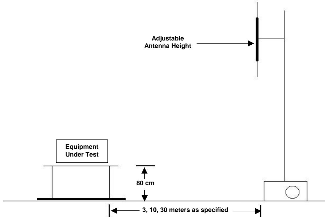
**Radiated Test Setup and Procedure - cont'd**
