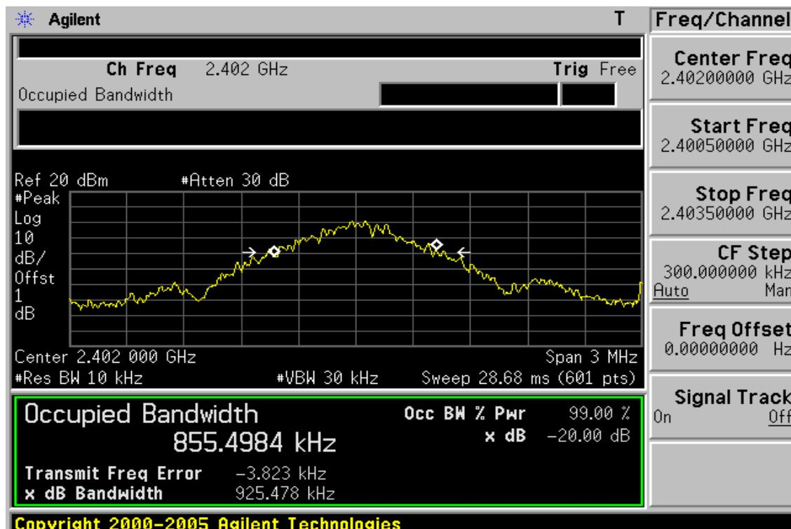
**20dB Bandwidth Test Data CH-Mid**
