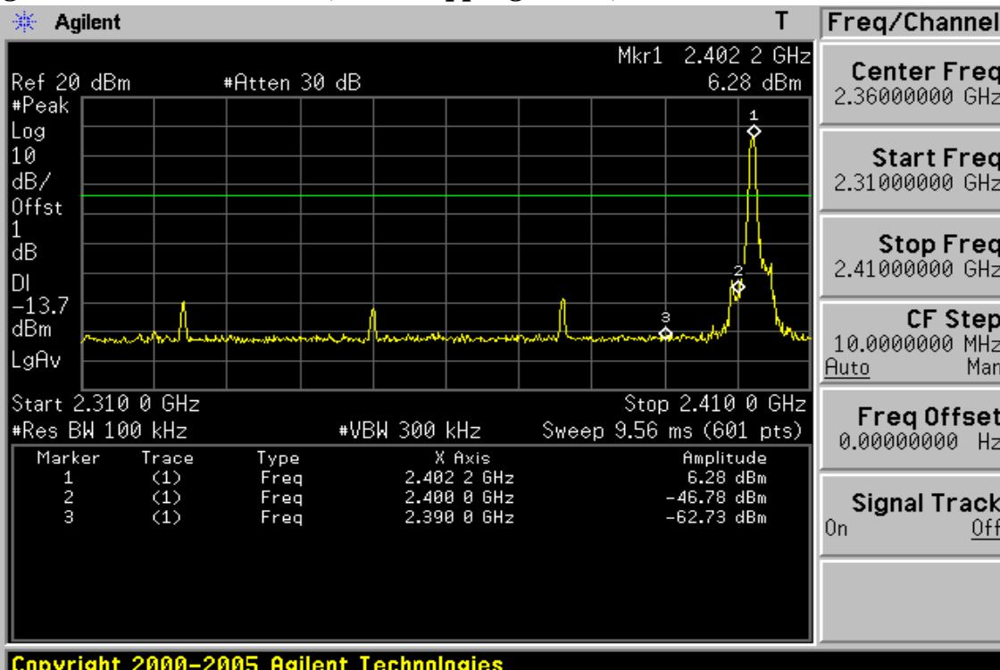
**Band Edges Test Data CH-High (Non-Hopping Mode)**
