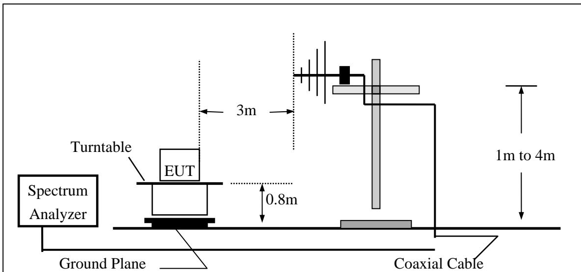
**(B) Radiated Emission Test Set-UP Frequency Over 1 GHz**
