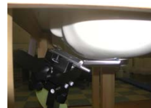
Fig. 14 Head SAR Test Setup
