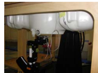
Fig. 15 body SAR Test Setup with Holster
