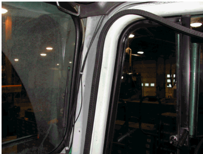
Figure20 Running of Antenna Cables Above Passenger Door Down to Dashboard
