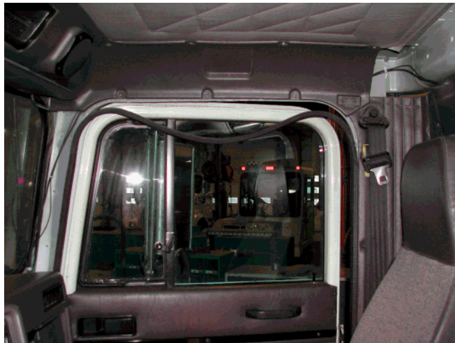
Figure19 Running of GPS and WAN Antenna Cables Through the Cab
