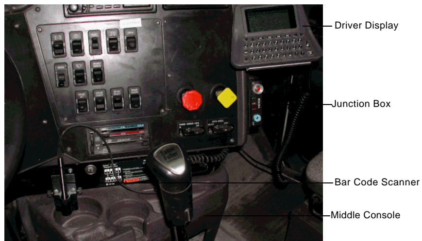
Figure28 Front View of the Complete Installation of the Driver Display, Junction Box and Bar Code Scanner
