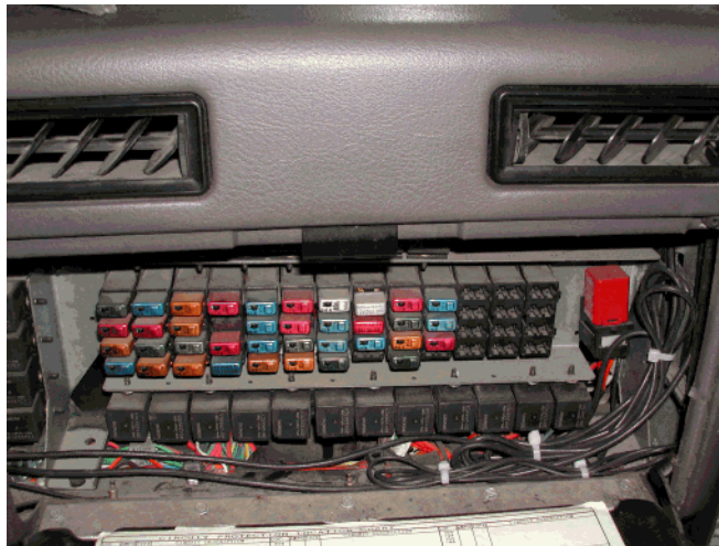
Figure21 Antenna Cables Behind the Glove Compartment and in Front of the Fuse Box
