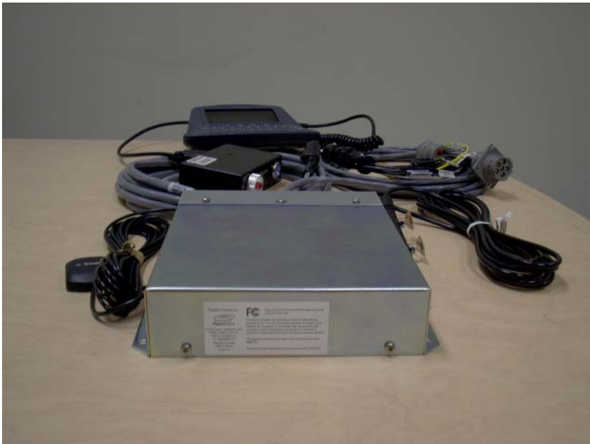
Photograph 4 - 2: Rear view of the Fleetlink M1 OBC with Terminal.
