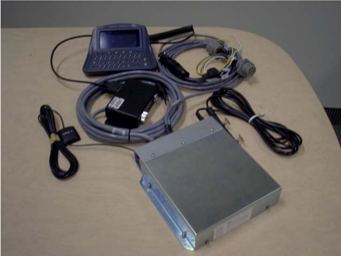
Photograph 4 - 5: Top view of the Fleetlink M1 OBC with Terminal.
