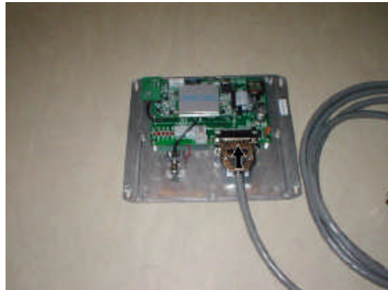
Figure 3-9 DB25 Cable connected inside the Access Point
