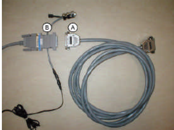
Figure 3-8 Splitter and DB25 Cable
