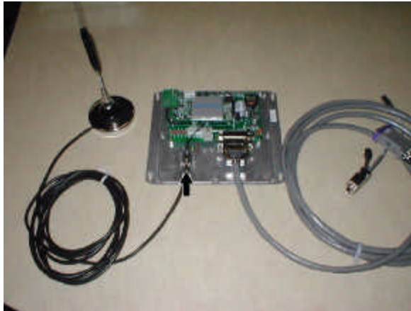
Figure 3-10 Antenna's coaxial cable connection
