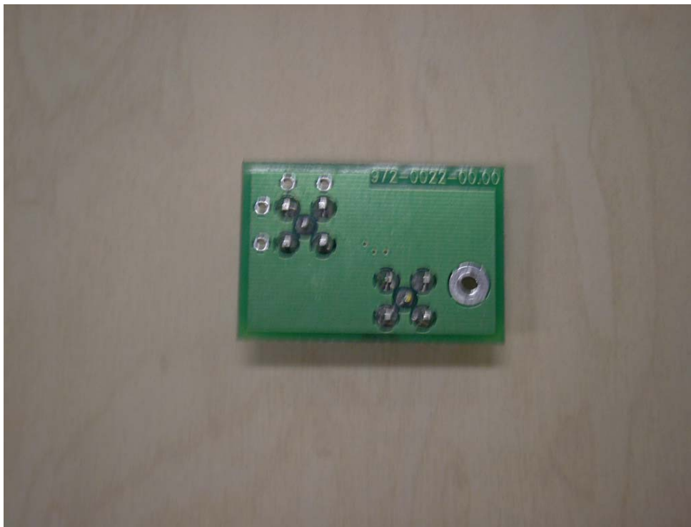
Photograph 5 - 7: Bottom Side of Filter.
