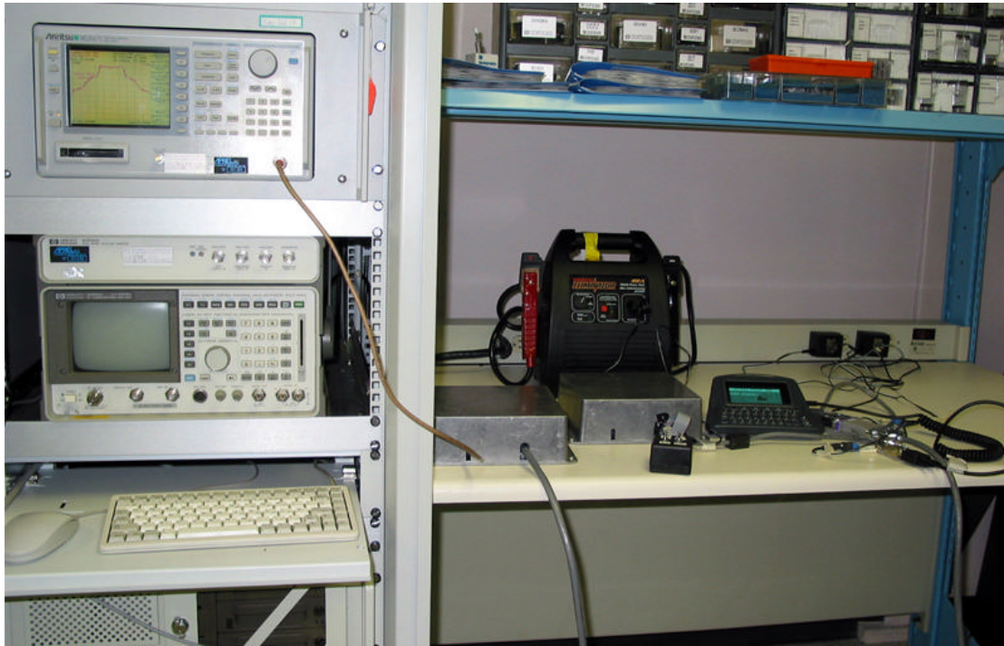
FleetMind – Access Point Spurious Emissions from Transmitter - Conducted Frequency Range: 9KHz – 10GHz
