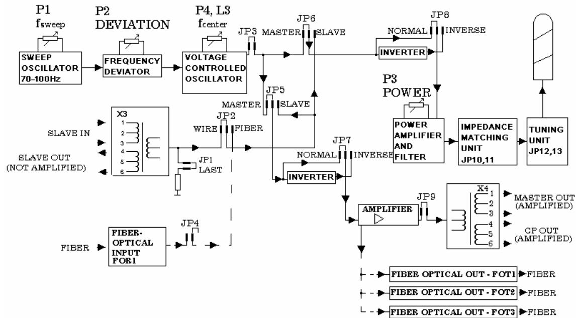
The above figure shows the schematic diagram of the transmitter circuit. Functions of the individual blocks are:
