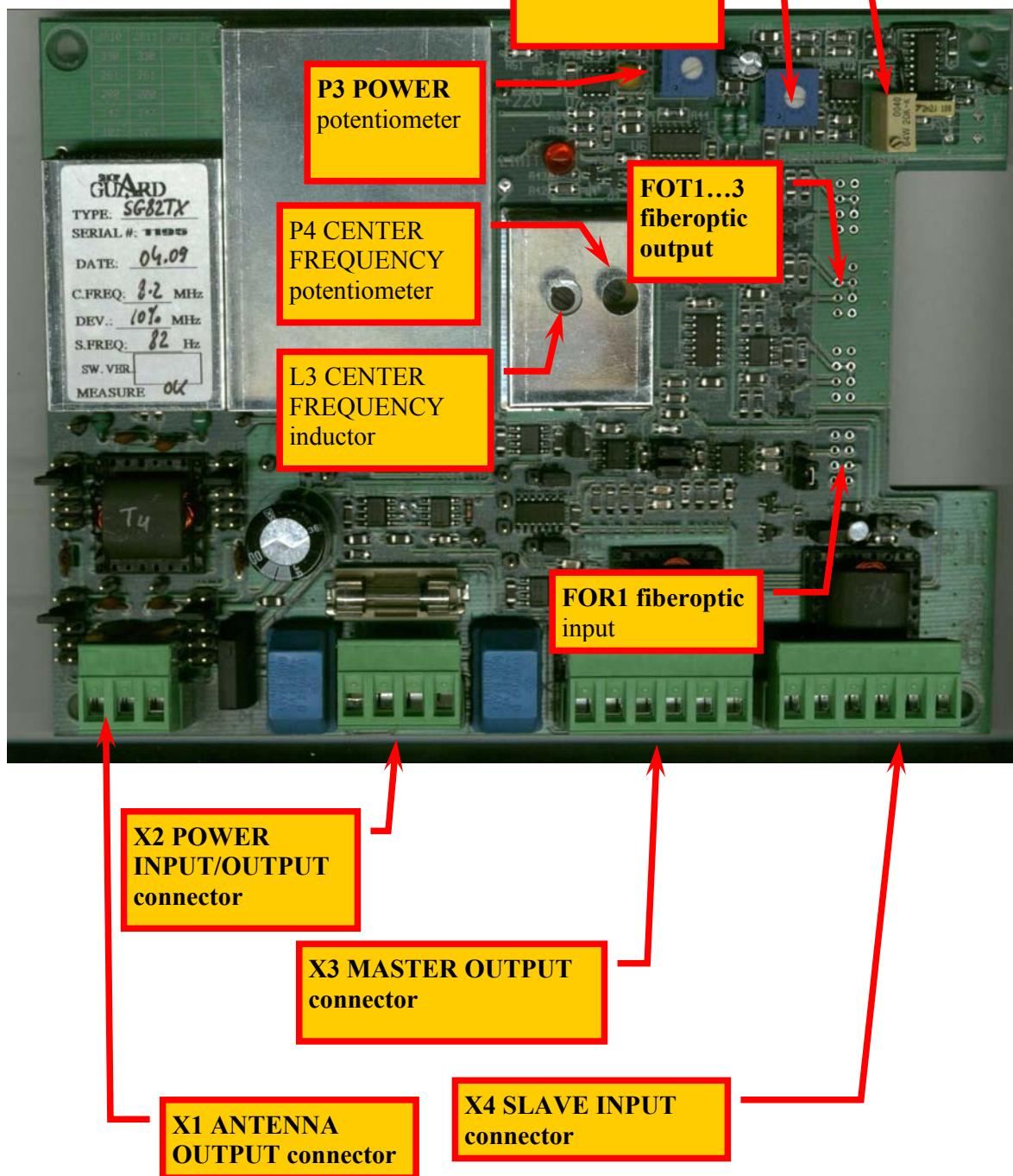
The photo on the last page shows SG82TX version REV3.0. The most important connectors, jumpers, potentiometers, as well as the optical transmitter and receiver are shown in picture.
