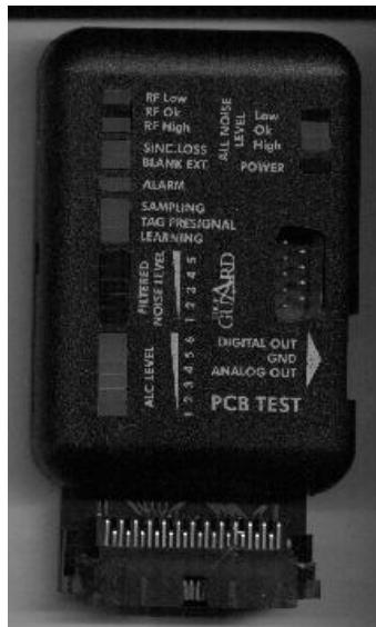
The test box connects to the X6 connector of the receiver board. The receiver board can be fitted even if the receiver board is operating. It provides help for testing and setting of the system delivered with factory set boards. The LEDs indicate the following (from up to down):
