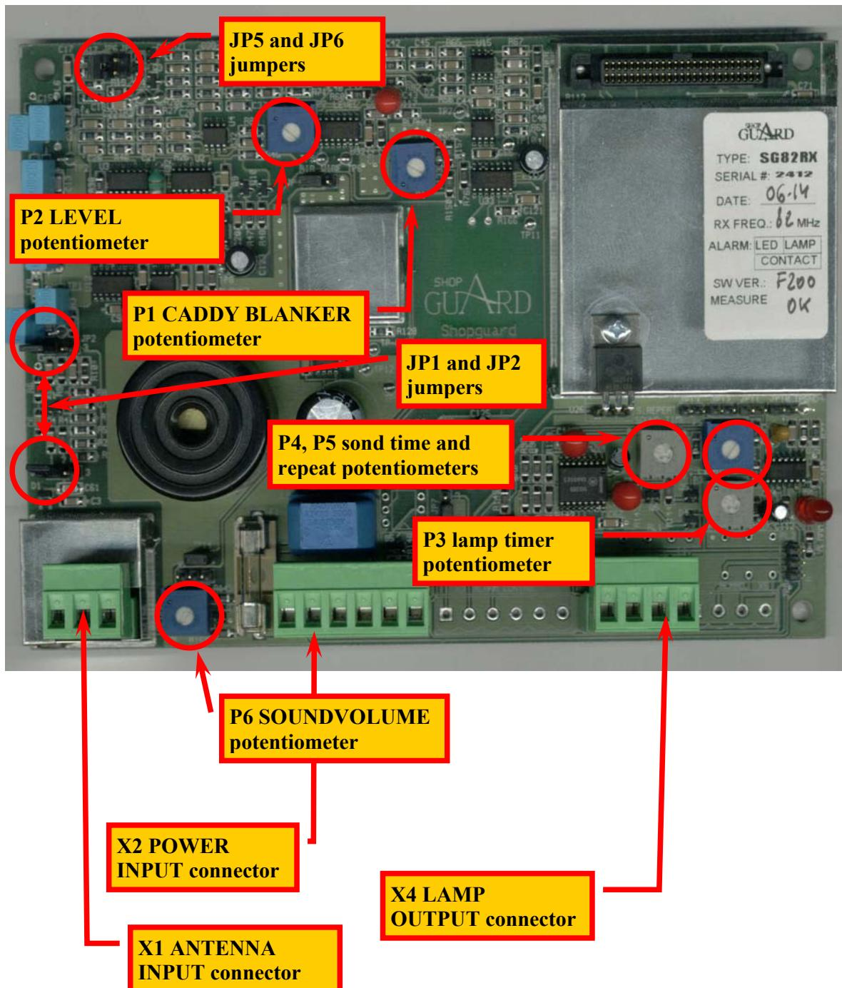
You can see the receiver board on this picture. On the datasheet are some important information for you: type, serial number, date, centre frequency (8.2MHz or 10MHz), software version. If you find problems with the board or the system, please send us these information.
