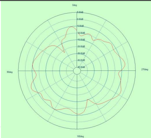
Free Space GAIN TOTAL (2440MHz) - XY cut
