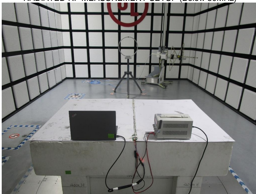
RADIATED RF MEASUREMENT SETUP (Below 30MHz)
