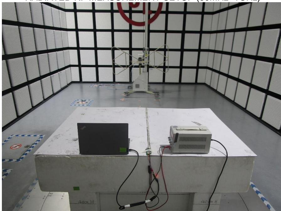
RADIATED RF MEASUREMENT SETUP (Below 30MHz)
