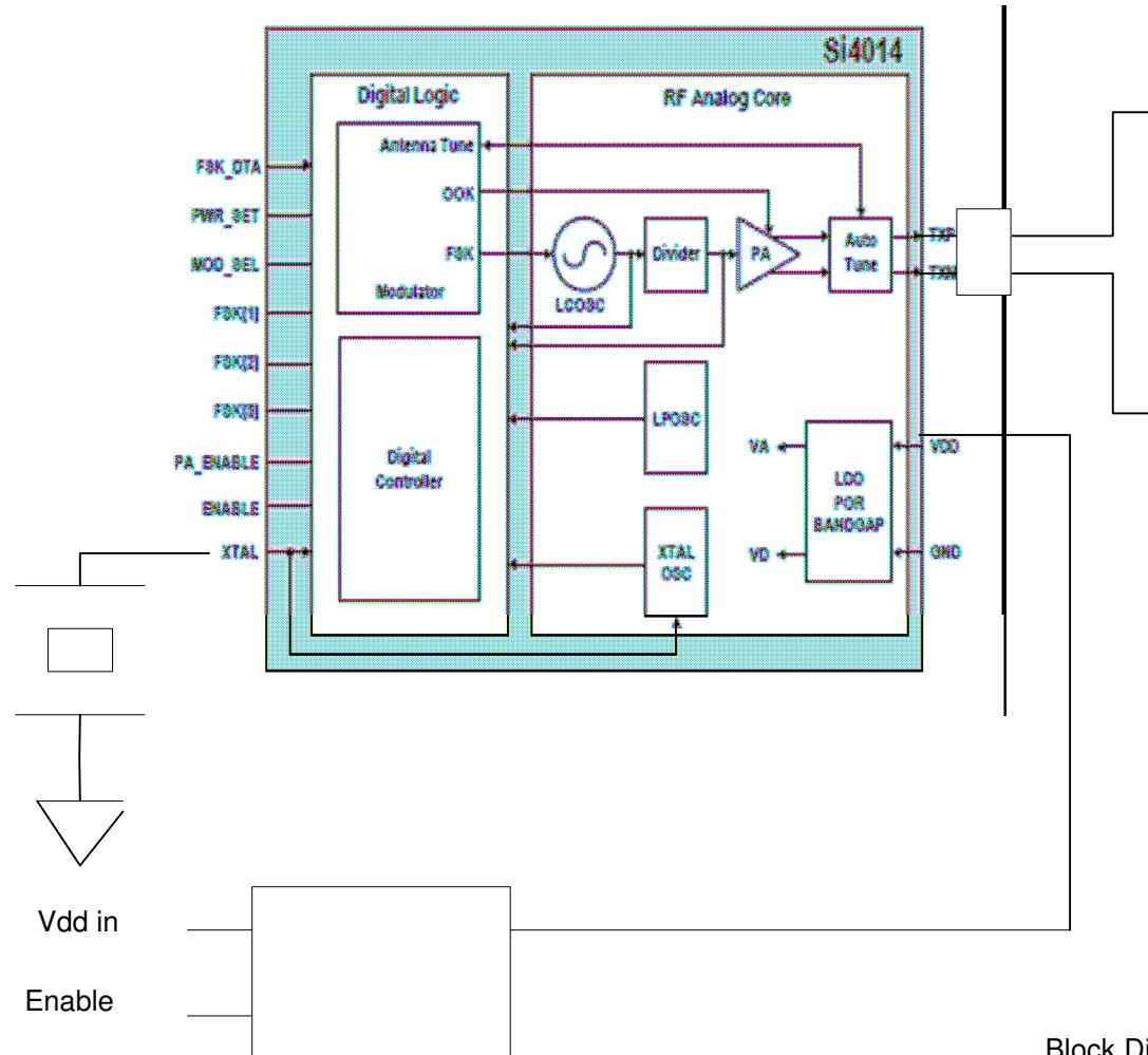
Block Diagram FSK Module
