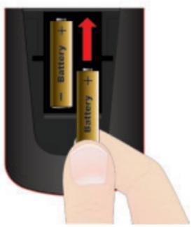
Insert 2 AA batteries, making sure to match the plus (+) ends with the plus markings on the battery case.
