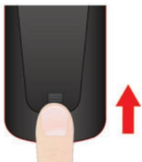
Push the tab toward the top of the remote to release the battery door latch and then lift the battery door from the remote.
