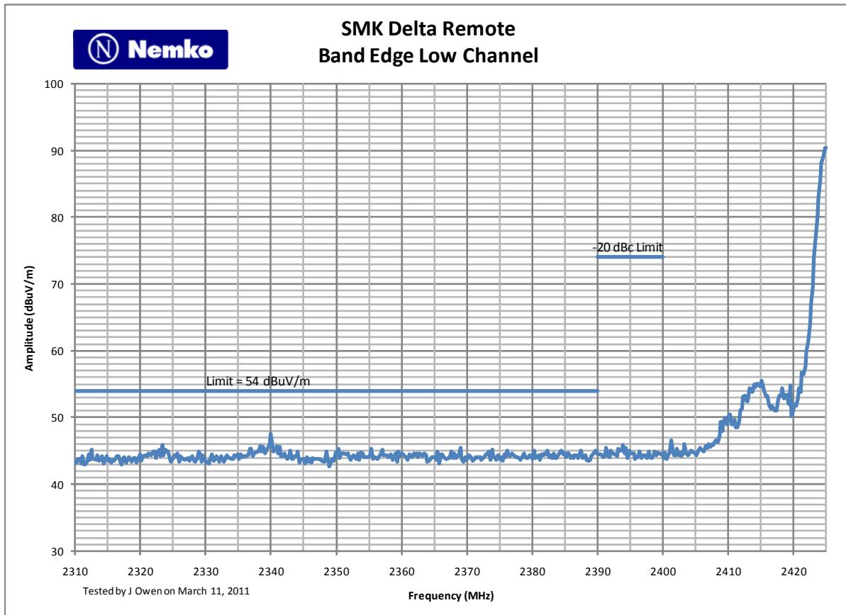
Low Channel 2425 MHz (Peak Measurement Corrected)
