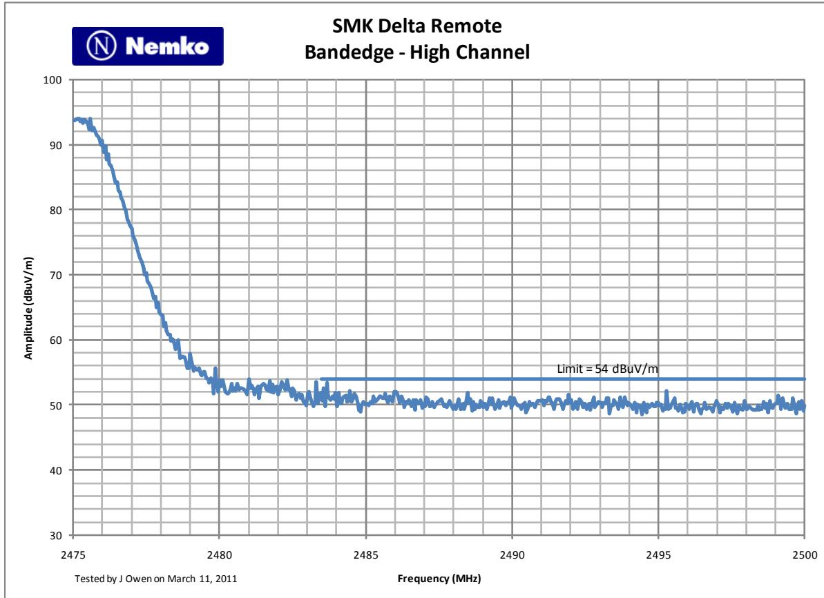
High Channel 2475 MHz (Peak Measurement corrected)
