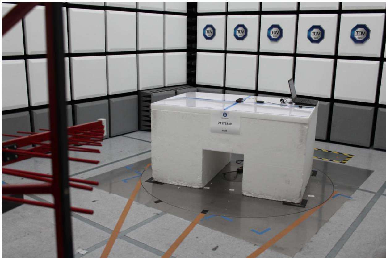
**Radiated Emissions Test Setup (30MHz to 1GHz)**
