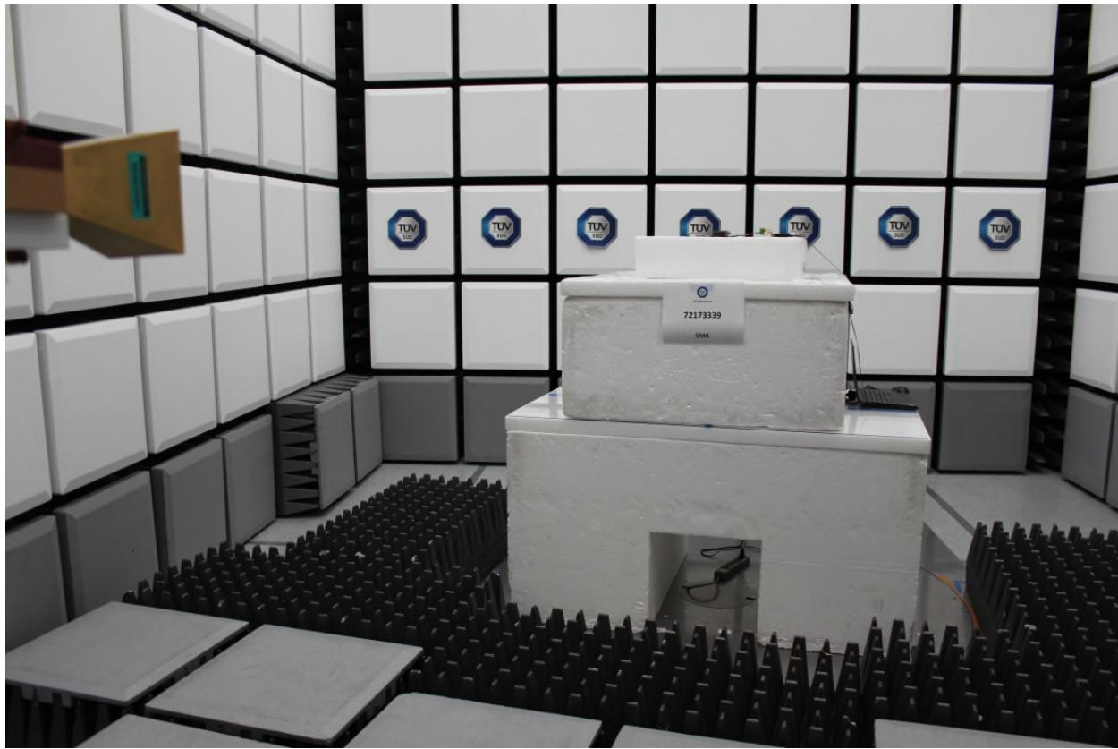
**Radiated Emissions Test Setup (18GHz TO 26GHz)**
